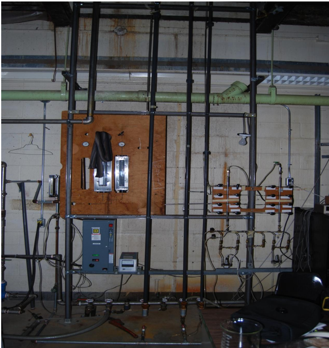
Figure 4.3 View of the test section and pressure transducers tubing
