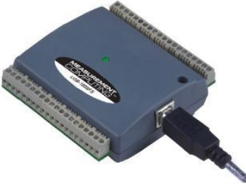
Figure 4.14 USB-based DAQ module with 8 analog channels of 16 bit resolution
