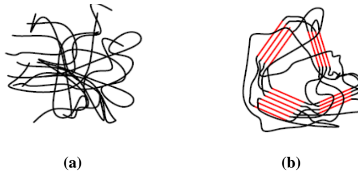
Fig. 7 Morphology of (a) amorphous and (b) semicrystalline polymer in the solid state
