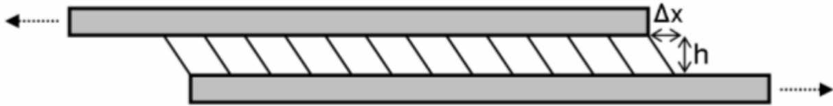
Figure 6.2: Schematic representation of shear strain. Grey portion represents each lamellae and the diagonal lines connect each lamellae represent the inter-lamellar matrix. Thickness of the inter-lamellar matrix ( h ) was assumed to be approaching zero, thus displacement ( \Delta x ) was of interest rather than shear strain. Arrows indicate direction of displacement.
