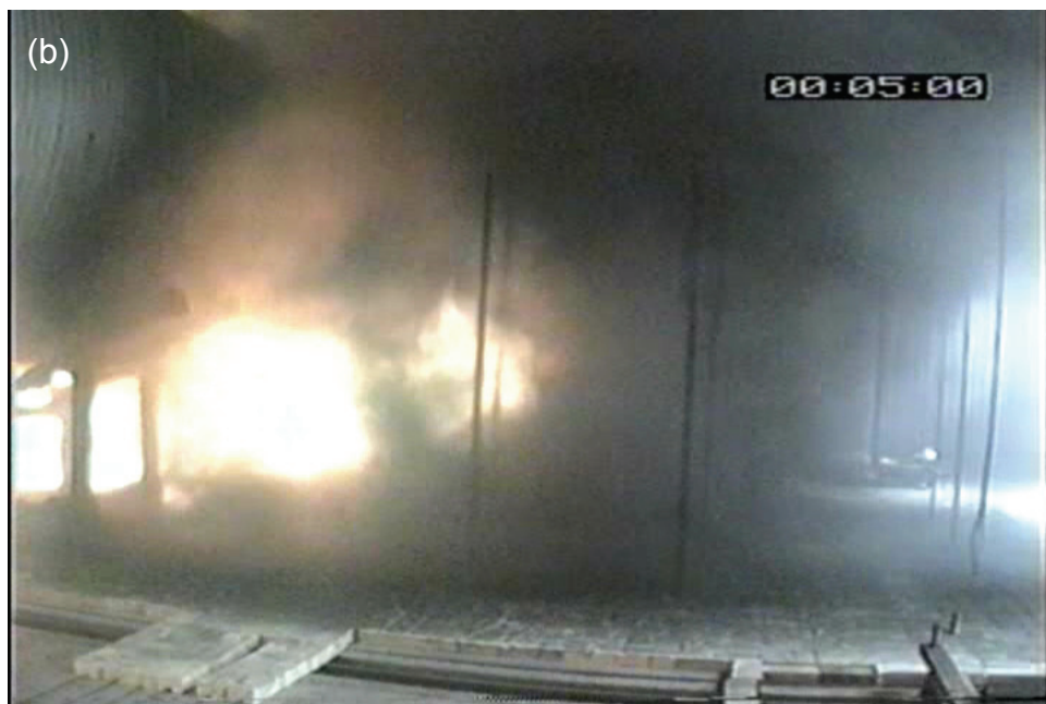
Figure 5.31: Typical video frames showing fire in 7 m/s wind, (a) upwind of blocking object, (b) downwind of blocking object
