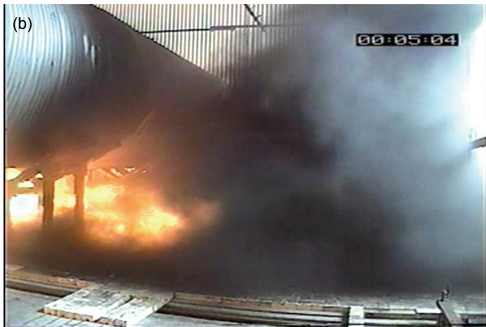
Figure 5.51: Typical video frames showing fire in 13 m/s wind, (a) upwind of blocking object, (b) downwind of blocking object
