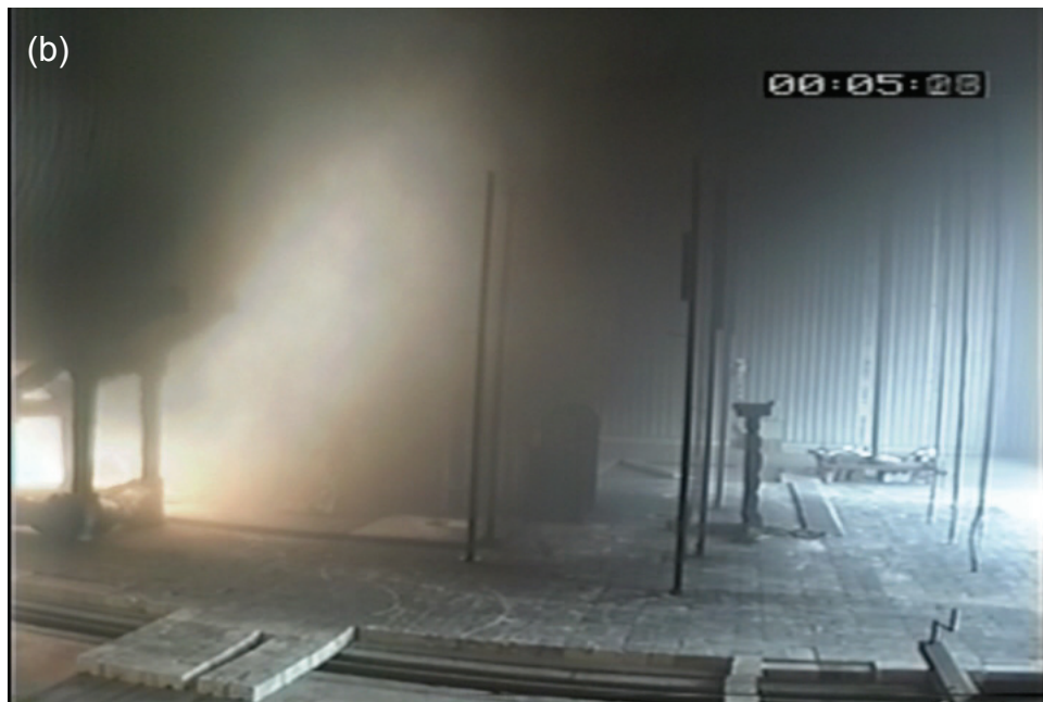
Figure 5.22: Typical 60-frame time-averaged images showing fire in 5 m/s wind, (a) upwind of blocking object, (b) downwind of blocking object
