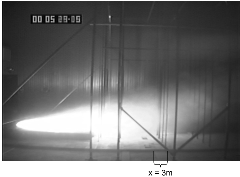
Figure 4.20: Typical 60-frame time-averaged image showing profile view of fire in 5 m/s wind
