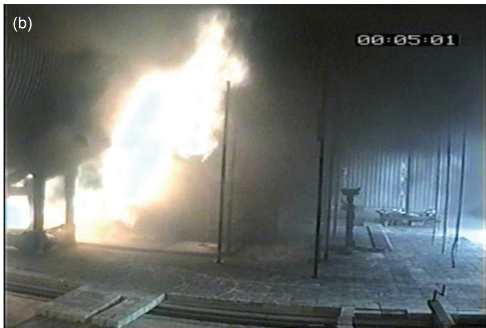
Figure 5.21: Typical video frames showing fire in 5 m/s wind, (a) upwind of blocking object, (b) downwind of blocking object
