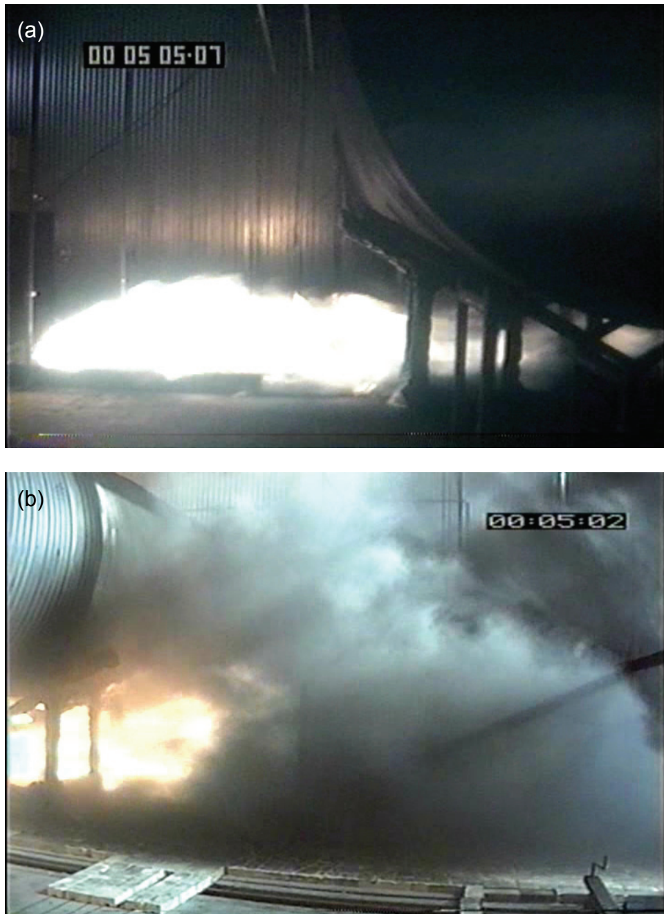
Figure 5.41: Typical video frames showing fire in 10 m/s wind, (a) upwind of blocking object, (b) downwind of blocking object
