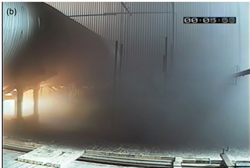
Figure 5.52: Typical 60-frame time-averaged images showing fire in 13 m/s wind, (a) upwind of blocking object, (b) downwind of blocking object
