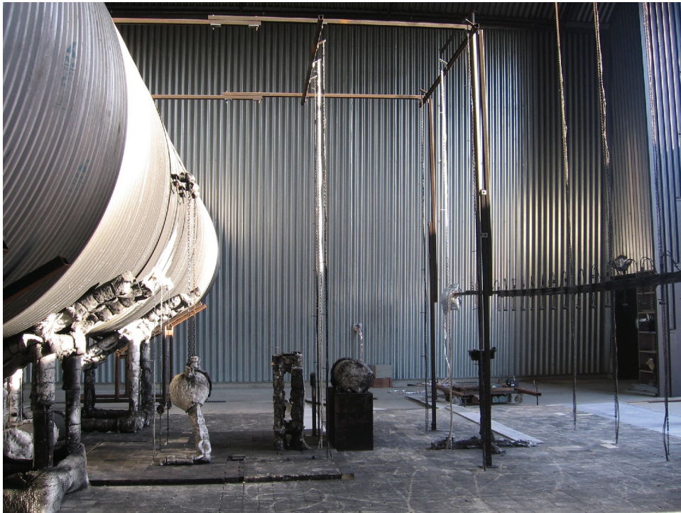
Figure 5.14: Photograph of experimental layout downwind of blocking object, side view
