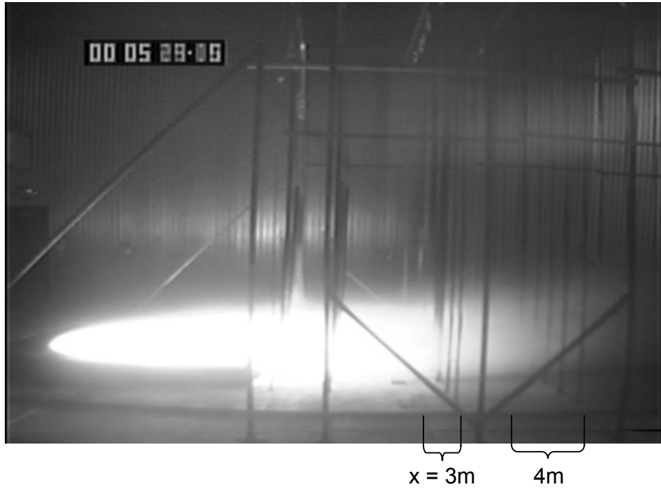
Figure 4.31: Typical 60-frame time-averaged image showing profile view of fire in 10 m/s wind
