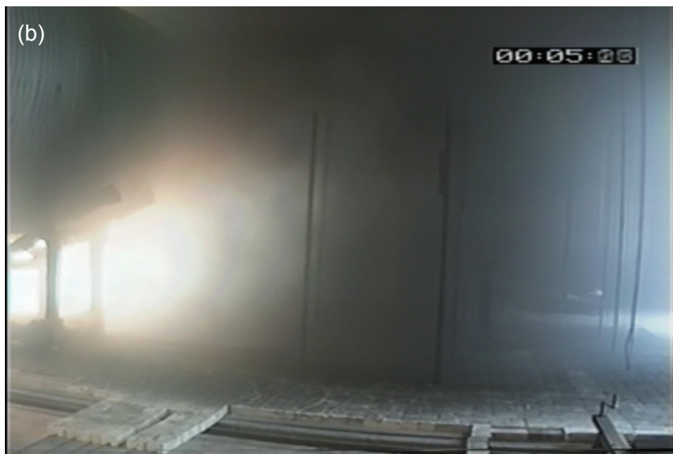
Figure 5.32: Typical 60-frame time-averaged images showing fire in 7 m/s wind, (a) upwind of blocking object, (b) downwind of blocking object
