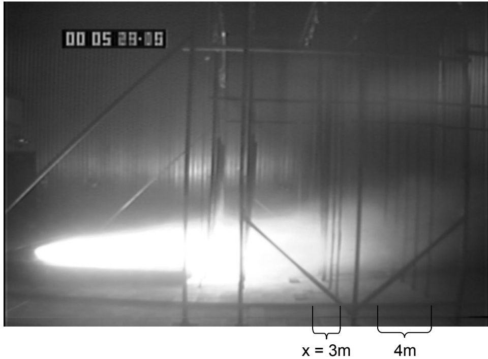
Figure 4.25: Typical 60-frame time-averaged image showing profile view of fire in 7 m/s wind
