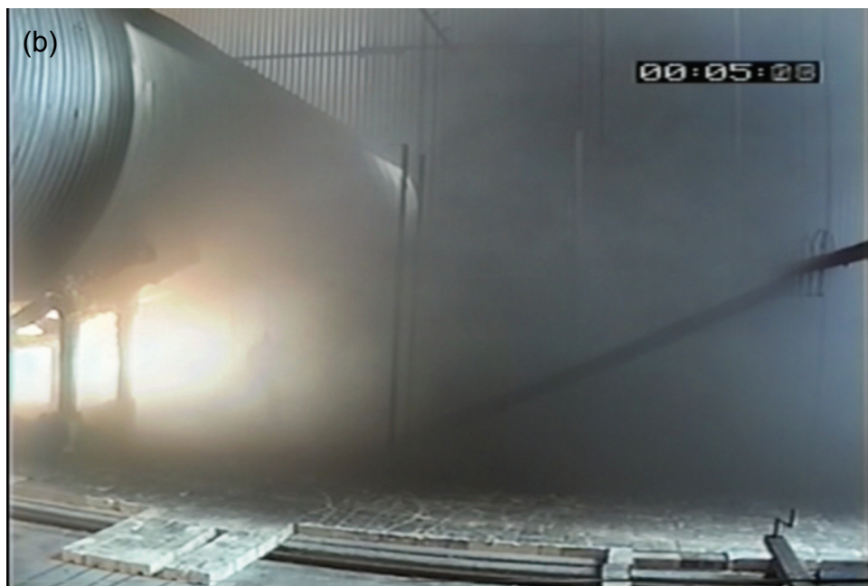
Figure 5.42: Typical 60-frame time-averaged images showing fire in 10 m/s wind, (a) upwind of blocking object, (b) downwind of blocking object
