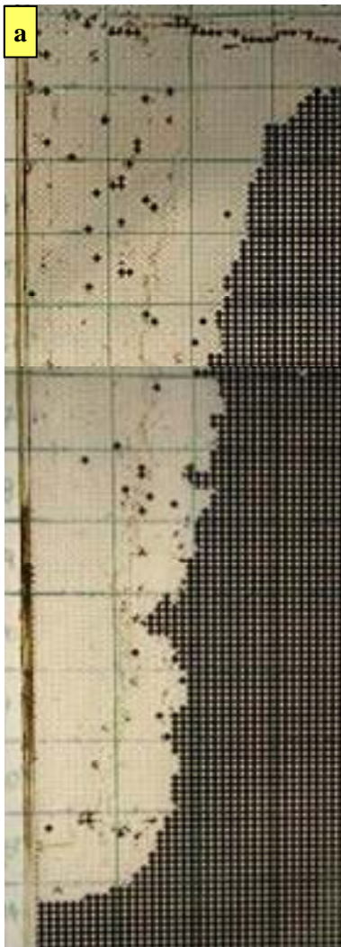
a) VAPEx showing no asphaltene precipitation in a glass micromodel
