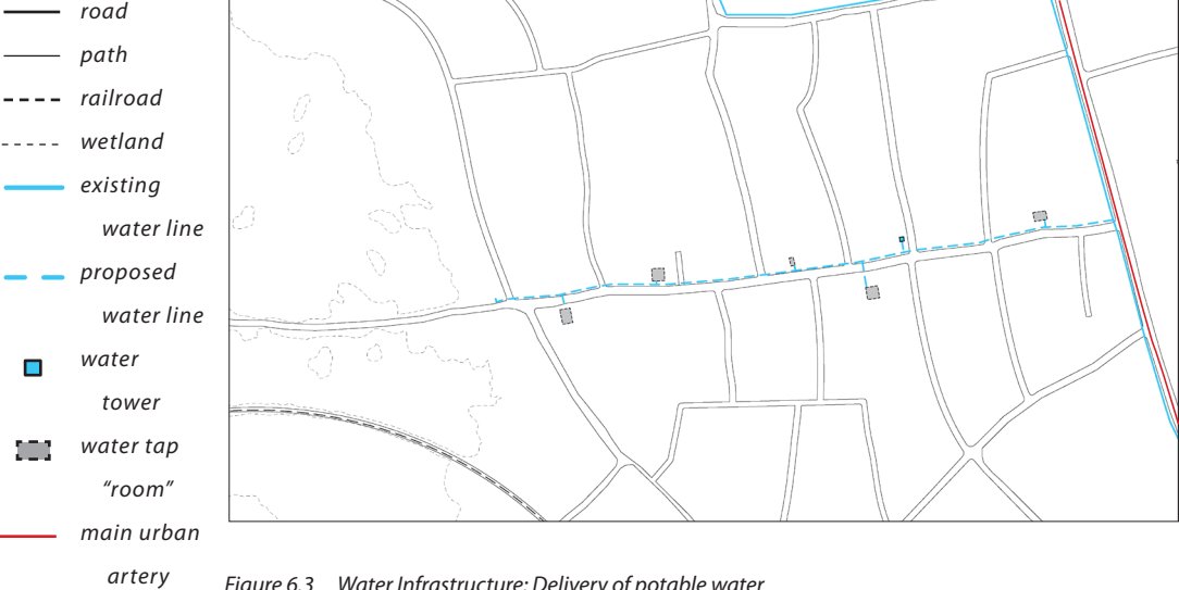
Figure 6.3 Water Infrastructure: Delivery of potable water
