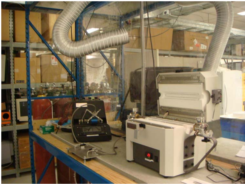
Figure 3.4: The photograph of a typical CVD system in our lab. It has the computer controlled gas flow system, the tube furnace to heat the reaction chamber, and the quartz tube reactor to hold the CVD synthesis.
