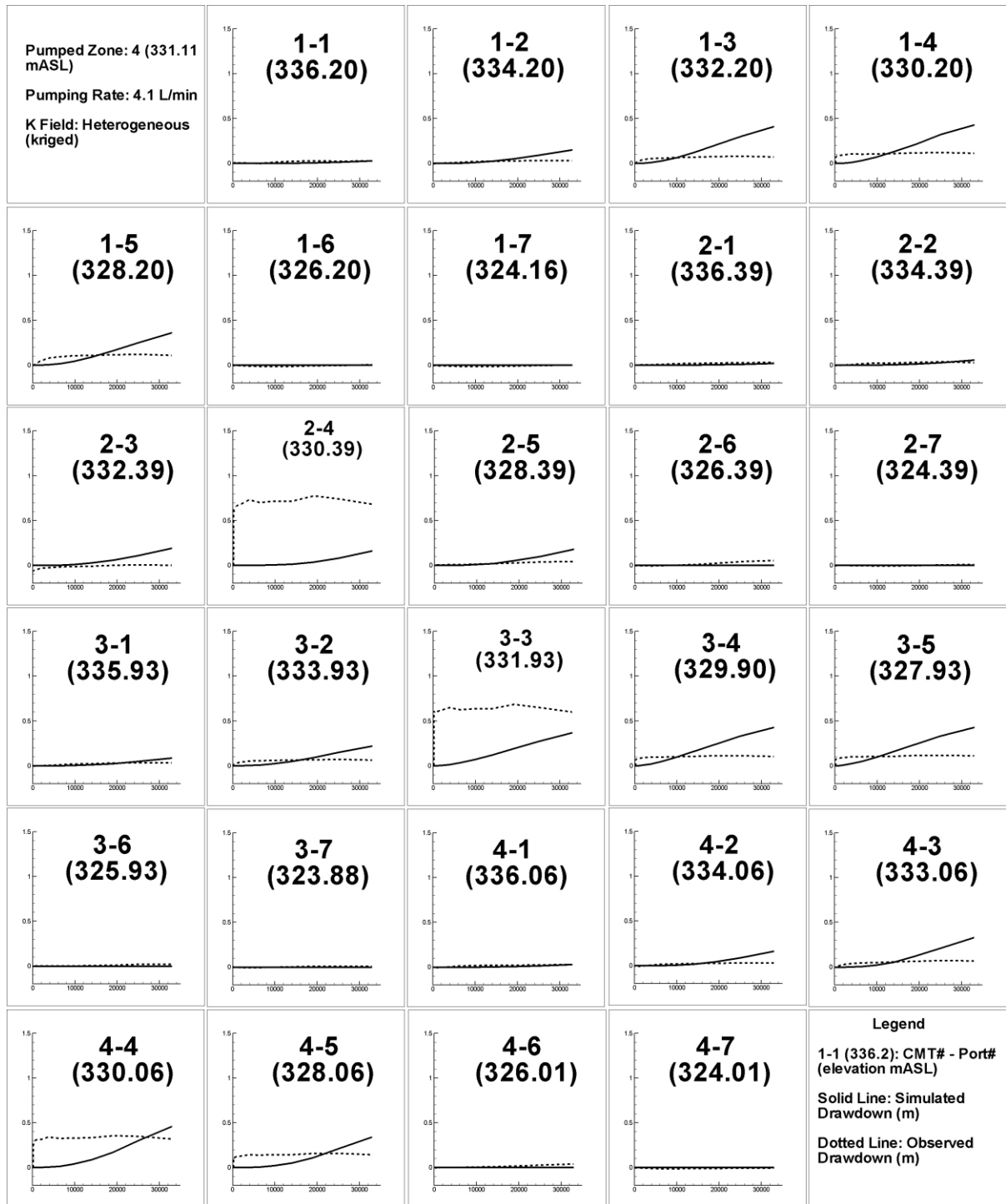
Figure A 26 Zone 4 HGS simulation results (heterogeneous kriged empirical equation data case). X-Axis is time in seconds and Y-Axis is drawdown in metres.
