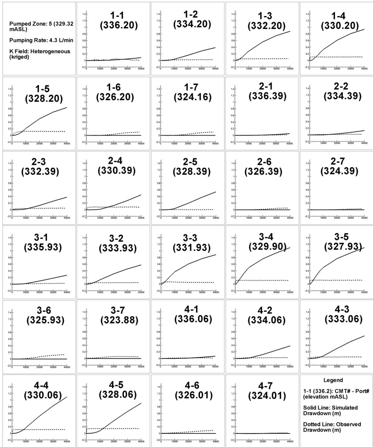
Figure A 32 Zone 5 HGS simulation results (heterogeneous kriged empirical equation data case). X-Axis is time in seconds and Y-Axis is drawdown in metres.
