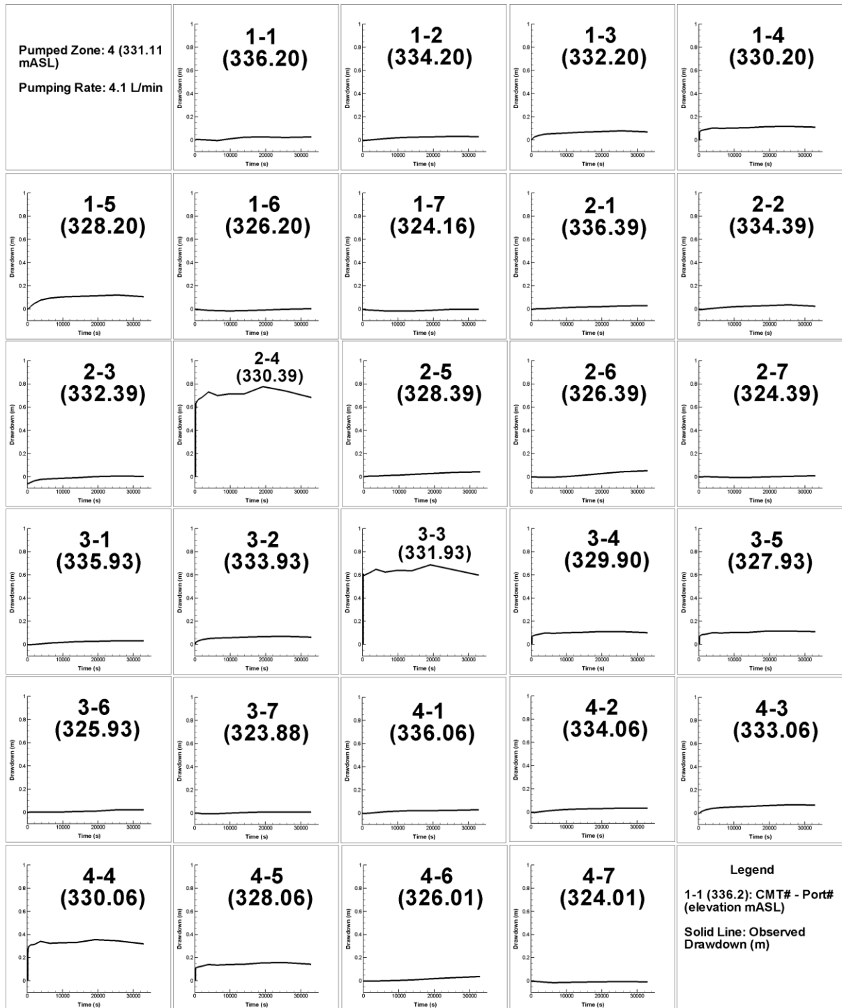
Figure 3.13 Drawdown observations in each CMT port during the Zone 4 pumping test. Time (s) is on the X-Axis and drawdown (m) is on the Y-Axis.
