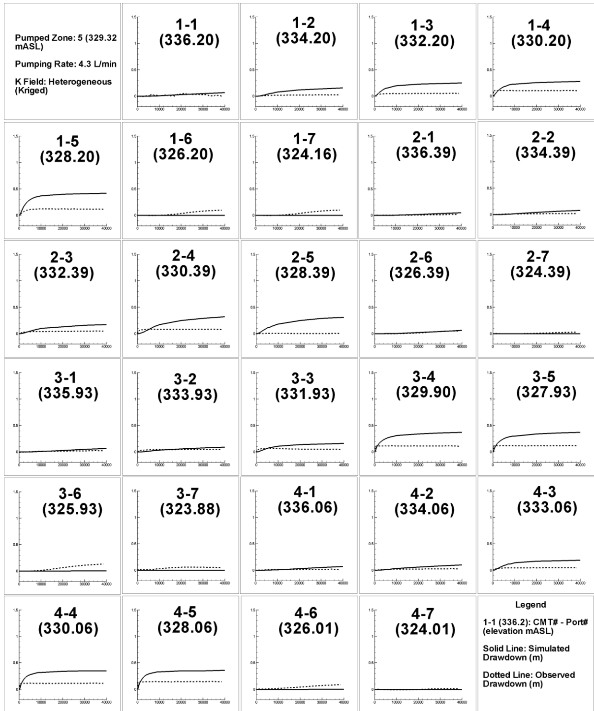
Figure A 31 Zone 5 HGS simulation results (heterogeneous kriged permeameter data case, tabulated S_s values). X-Axis is time in seconds and Y-Axis is drawdown in metres.
