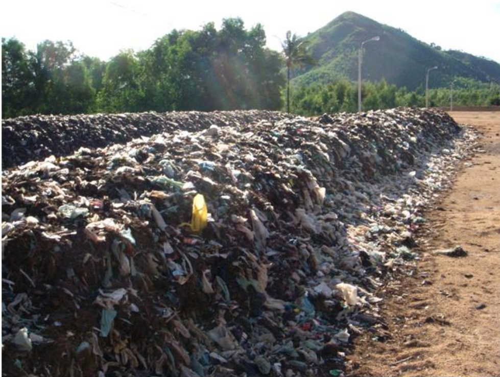
Photo 12 - Composting windrows at the Quy Nhon large-scale composting plant. Note the presence of significant amounts of contaminants due to the lack of source separation
