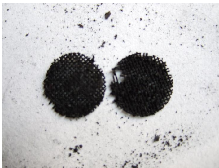
Figure 5-2: The visual of the screen with covering with tar after the experiment failed due to plugging.
