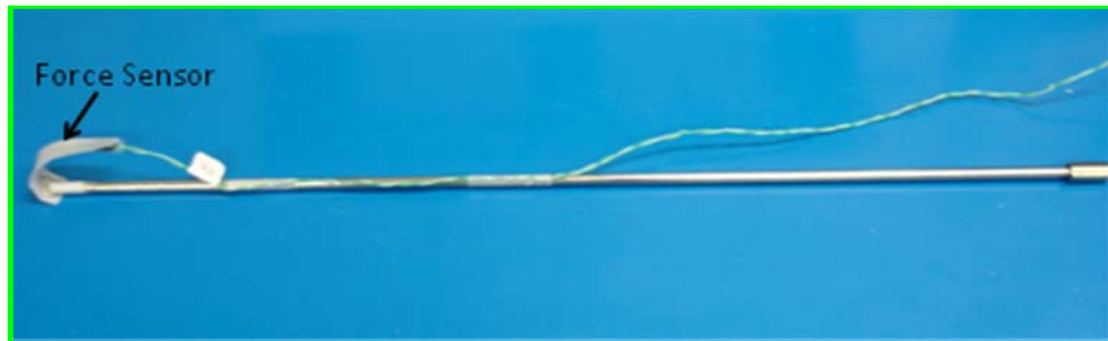
Figure 3: Laparoscopic probe with force sensor
