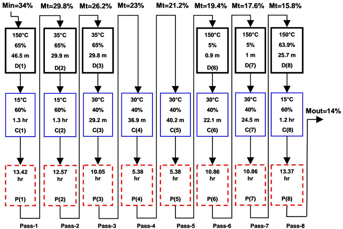
Figure 3.5 The optimal flowsheet of maximization of HRY with the ad hoc model from Case study 1.
