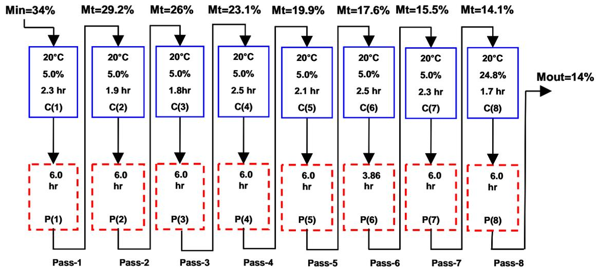
Figure 4.15. Optimum configuration of the synthesis problem using the theoretical models which minimize the energy objective function while maintains the quality of rice grain.
