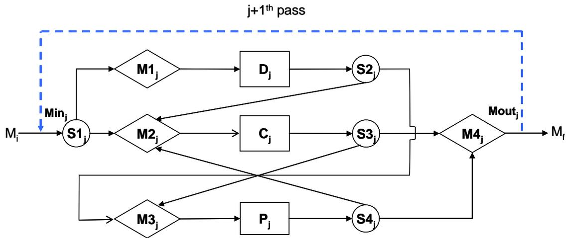
Figure 2.2. Five-alternative superstructure representation of synthesis of rice drying processes using theoretical models.
