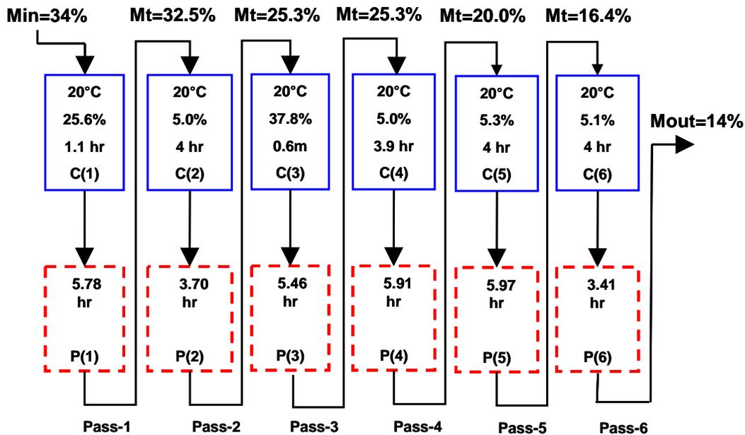
Figure 4.14. Optimum configuration of the synthesis problem with energy objective function using the theoretical model with 4 hr maximum cooling time allowed.
