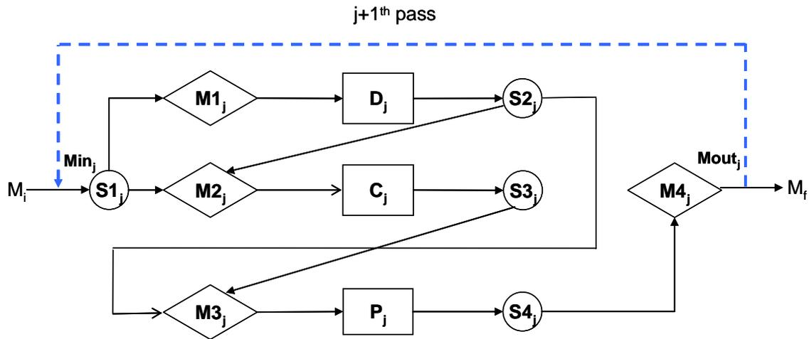
Figure 2.1. Three-alternative superstructure representation of synthesis of rice drying processes using empirical models.
