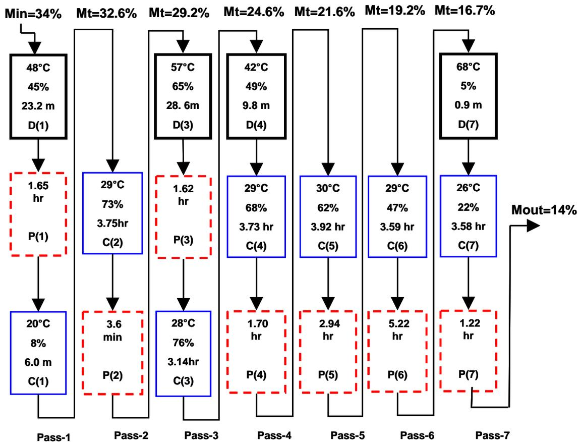
Figure 4.12. Optimum configuration of the synthesis problem with quality objective function using the theoretical model.
