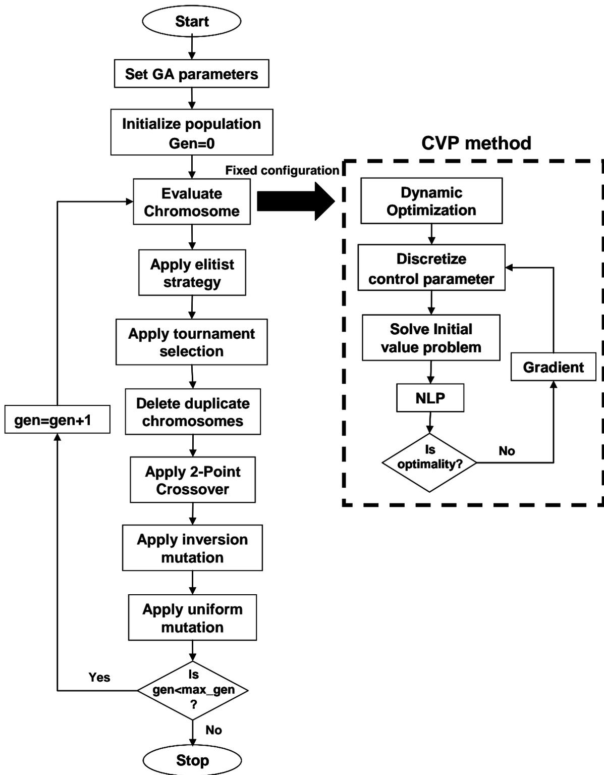
Figure 4.3. Algorithm structure of hybridization method.
