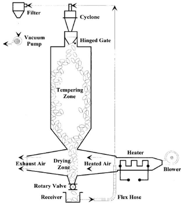
Figure 1.5. Re-circulating rice dryer with a drying and a tempering zone (Shei and Chen, 2002).
