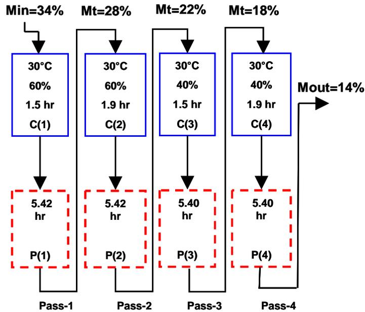
Figure 3.12. The optimal flowsheet of minimizing of energy consumption from Case Study 3.
