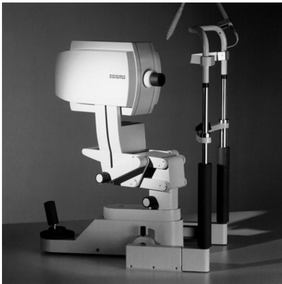
Figure 1.4 Photograph of the Heidelberg Retina Flowmeter. Laser head of the instrument mounted on a table and attached to a chin rest.
