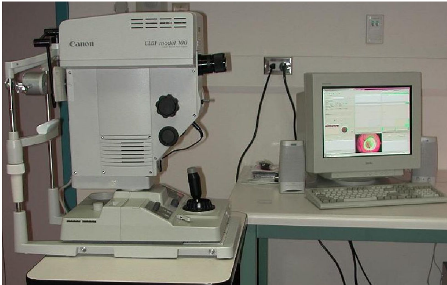
Figure 1.6 Photograph of the Canon laser blood flowmeter (model 100).
