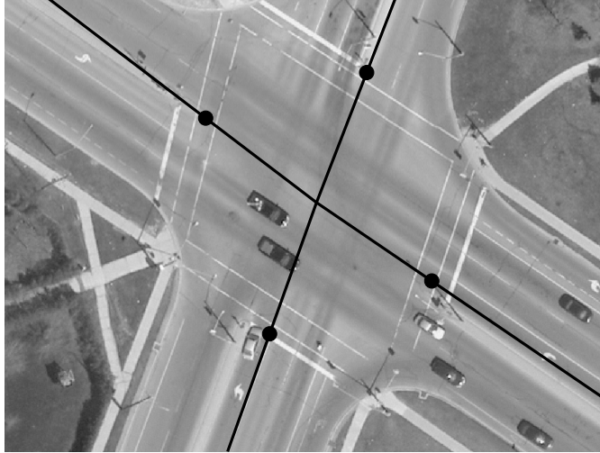
Figure 4.4: A model of intersection road marking locations, generated by knowing the center point of the intersection and the distance from the center point to the road markings.
