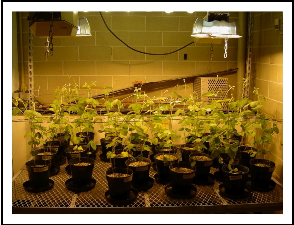
Figure 3.9: Soybean growth facility constructed within the Charles lab at the University of Waterloo. This set-up employed two high-pressure sodium bulbs, augmented by compact fluorescent bulbs and was capable of holding up to 30 pots simultaneously without cross-contamination
