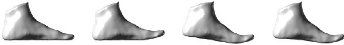
Figure 4-7 from left to right: Flat, Toespring Added, Heel Height Added, Mid Section Adjusted
