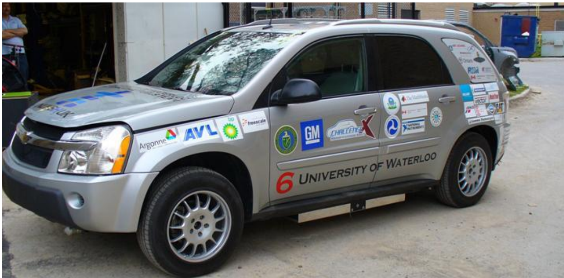
Figure 30 - Fuel Cell/Battery Hybrid Vehicle "Inukshuk"
