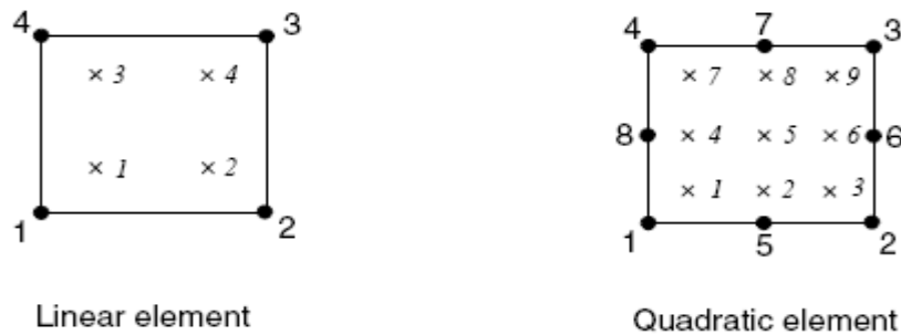
Figure 3.8: Integration points in fully-integrated, two-dimensional, quadrilateral elements (Abaqus User's Manual, 2007).
