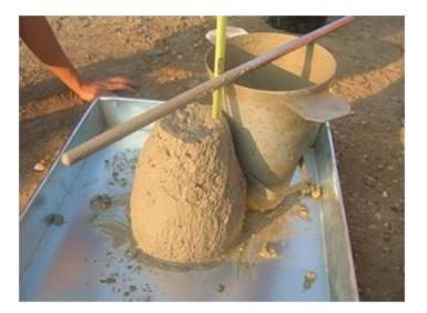
Figure 36: On Site Concrete Slump Testing
