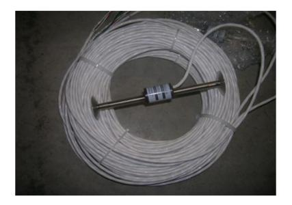
Figure 42: Vibrating Wire Asphalt Strain Gauge
