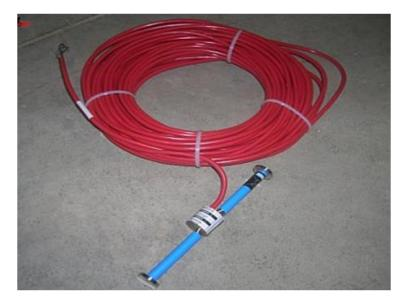
Figure 43: Vibrating Wire Concrete Strain Gauge
