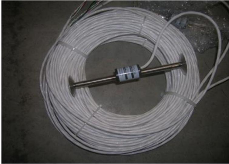
**Figure 42: Vibrating Wire Asphalt Strain Gauge**
