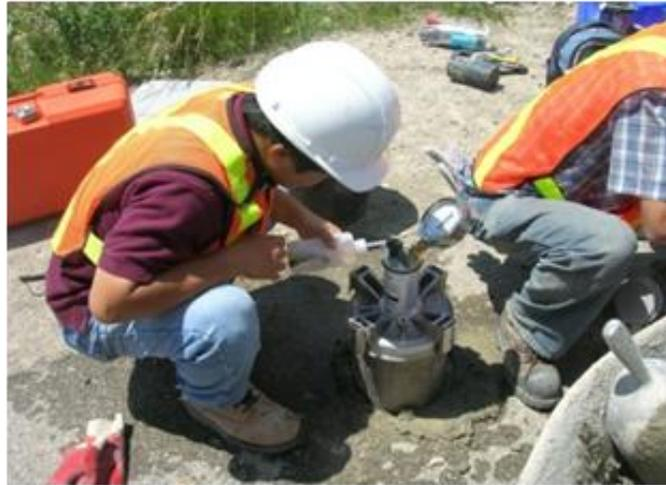
**Figure 20: On-site Concrete Air-Void Testing**
