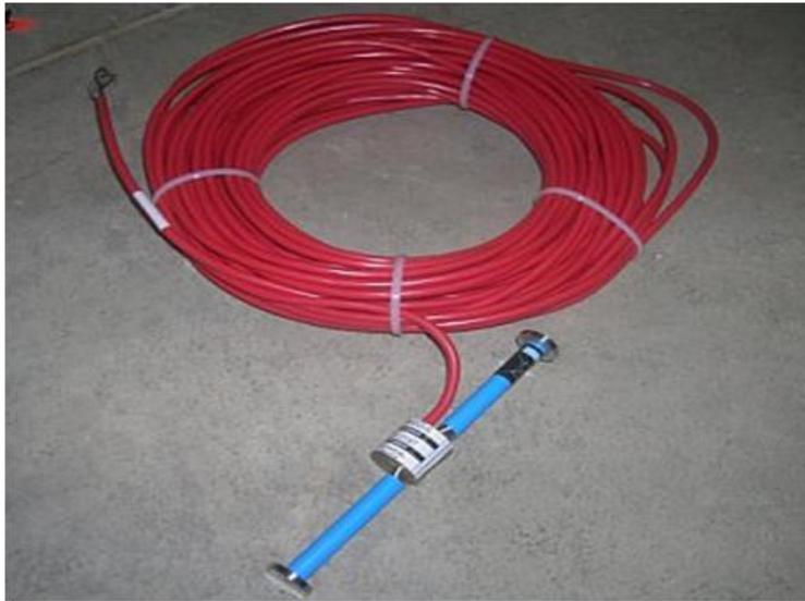
**Figure 43: Vibrating Wire Concrete Strain Gauge**
