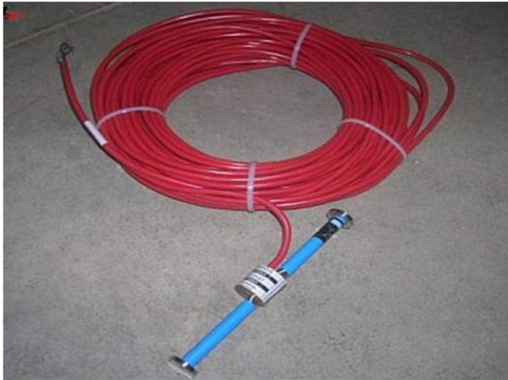
**Figure 43: Vibrating Wire Concrete Strain Gauge**
