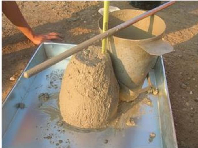
**Figure 36: On Site Concrete Slump Testing**
