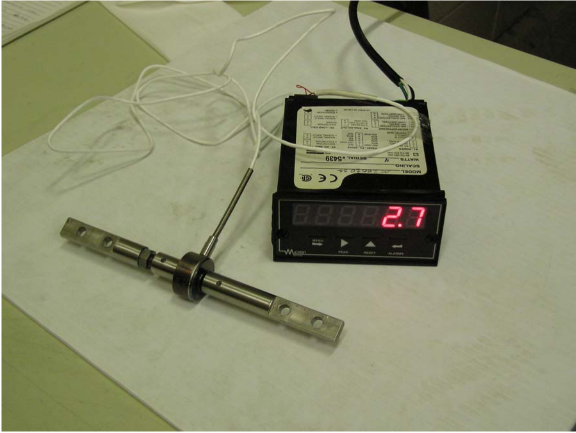
Figure 3.7: Load cell and digital display used for text fixture calibration.
