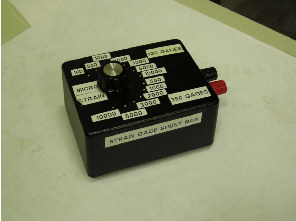
Figure 3.8: Strain gauge shunt box used for data acquisition calibration.
