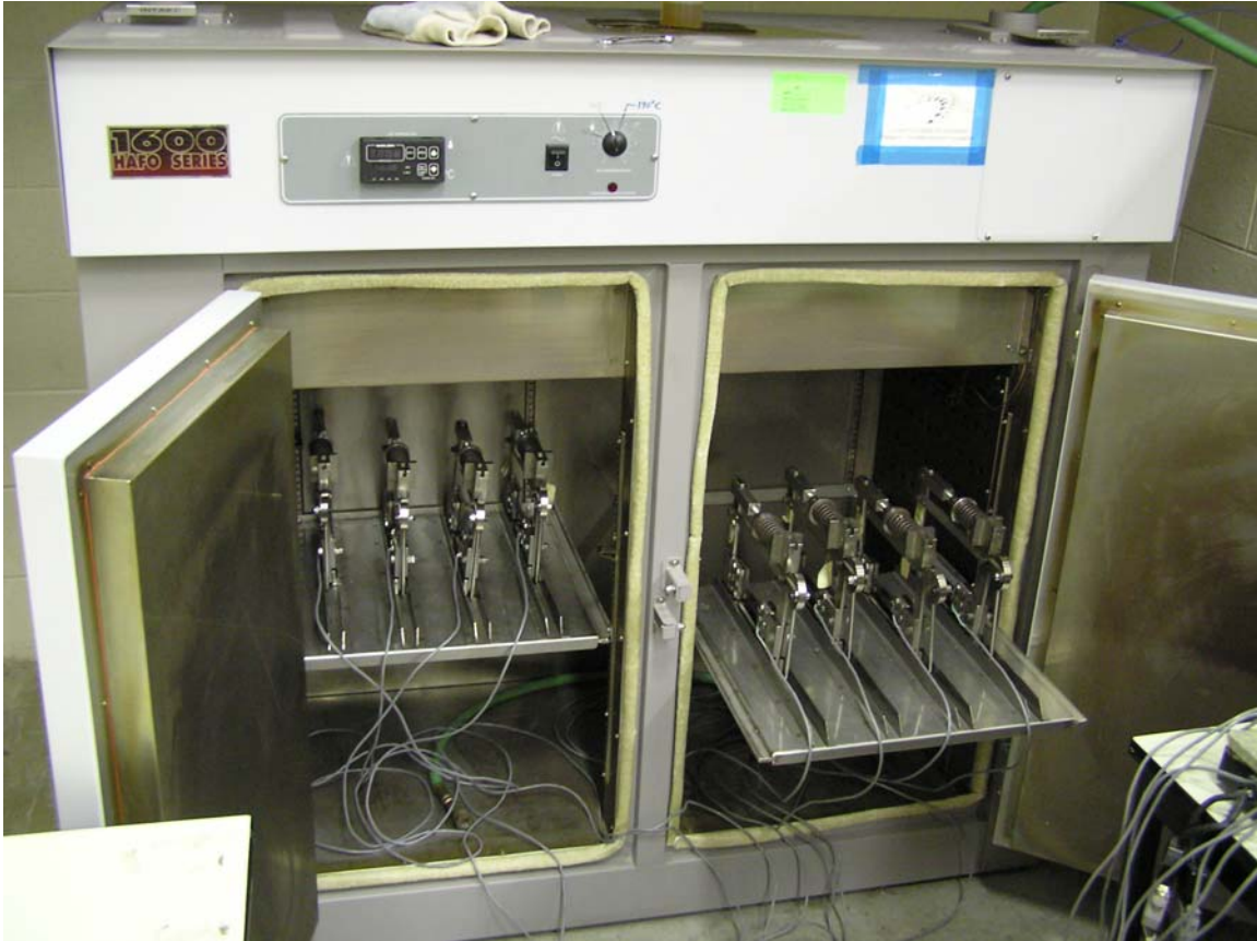
Figure 3.9: Oven used for creep testing.
