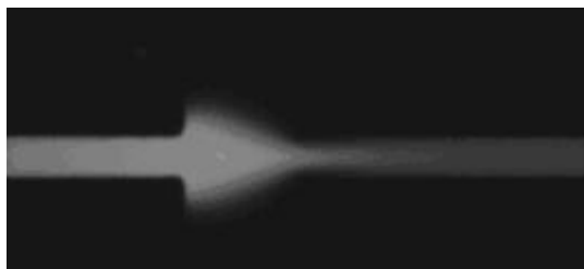
Figure 4-4 Focusing investigation with fluorescent dye. After focusing intersection. The fluorescent dye is focused almost at the center of the channel.
