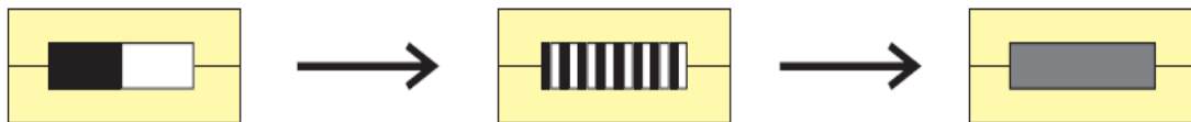
Figure 2-7 Schematic of the splitting by continuous geometric separation and reunion of fluid embodiments (laminar mixing)(WolfgangEhrfeld 2000).
