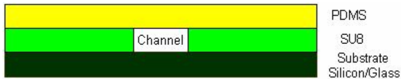
Figure 2-4 Illustration of PDMS-SU8-Silicon/Glass chip
