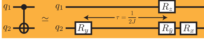
Figure 2.2: Implementation of a controlled-NOT gate in liquid state NMR. The CNOT is equivalent to a J-coupling evolution up to local operations.
