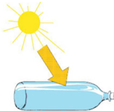
Figure 1.2: SODIS uses the UVA radiation and thermal energy from the sun to disinfect water (Solar Water Disinfection, 2002b)
