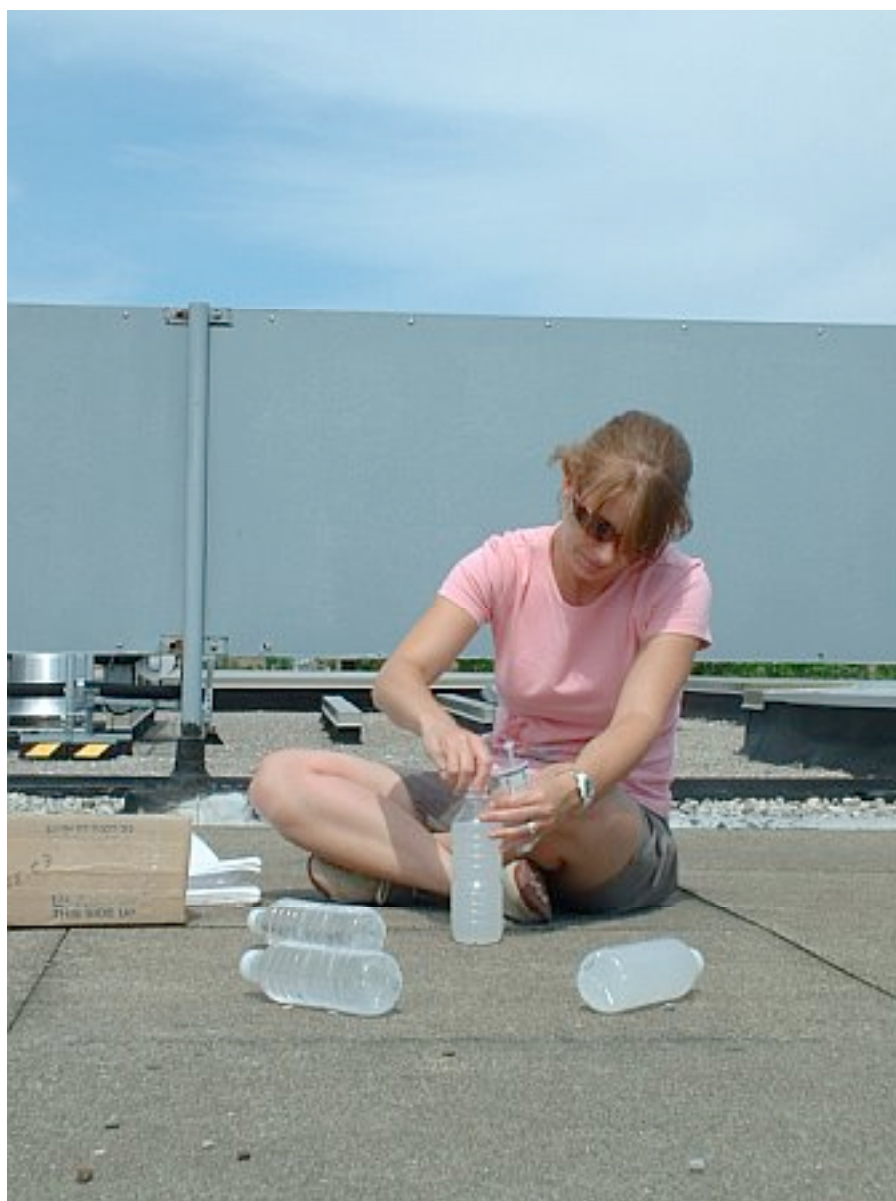
Figure 5.1: SODIS in action; bottles on the left were pretreated using the roughing filter, while bottles on the right contained unfiltered water (Waterloo, Ontario)
