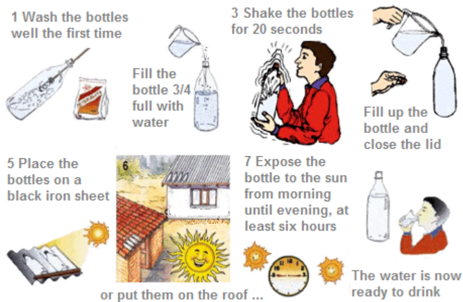
Figure 2.4: Depiction of the SODIS process (adapted from RCSI Research)
