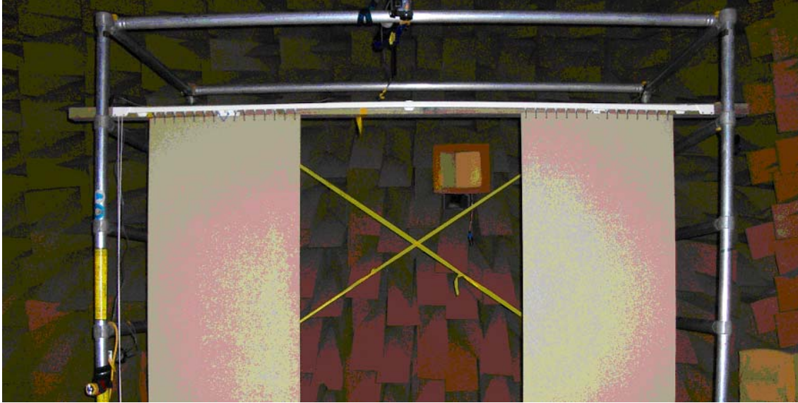
Figure 7.1 Experimental apparatus for aperture testing within the anechoic chamber.
