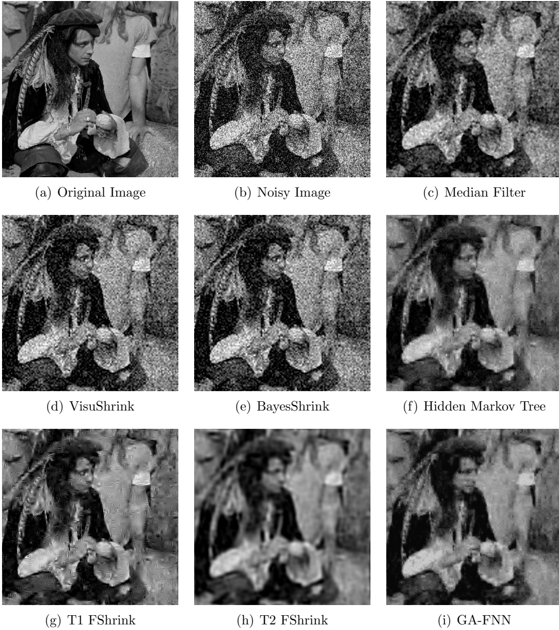
Figure 5.4: Results of “man” with Gaussian noise variance 0.05. From the point of human vision, median, VisuShrink and BayesShrink filters do not remove noise completely. T1 FShrink causes some artifacts. T2 FShrink and GA-FNN outperforms other algorithms, but T2 FShrink smooths the edges more.
