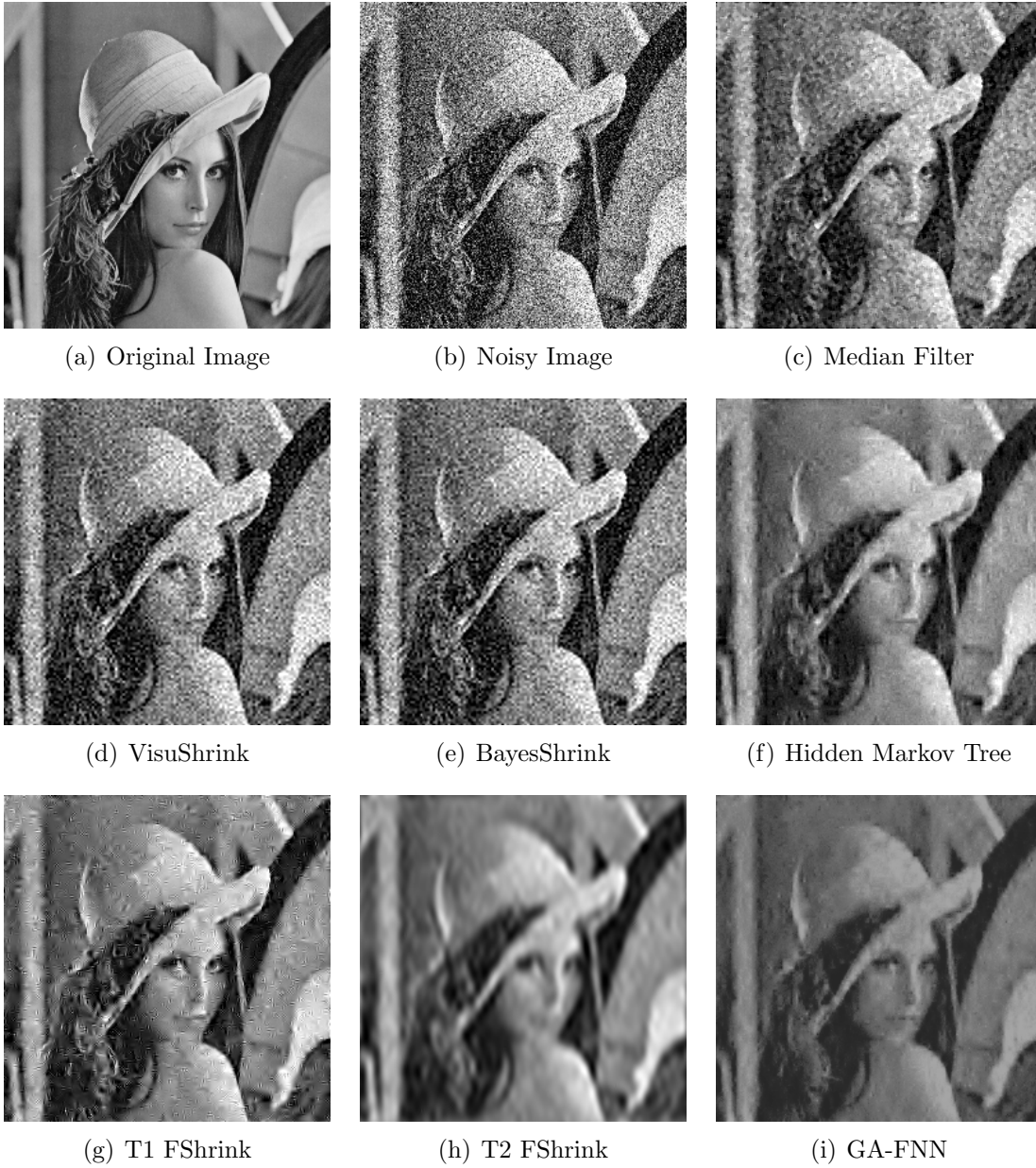
Figure 5.2: Results of “lena” with Gaussian noise variance 0.05. From the point of human vision, median, VisuShrink and BayesShrink filters do not remove noise completely. T1 FShrink causes some artifacts. T2 FShrink and GA-FNN outperforms other algorithms, but T2 FShrink smooths the edges more.
