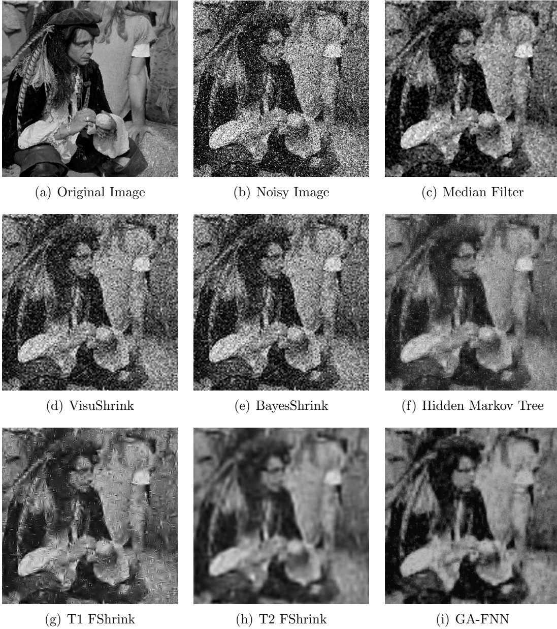
Figure 5.17: Results of “man” with Gaussian and Impulsive Noise (Both noise variance are 0.05). T2 FShrink and GA-FNN algorithms outperform other algorithms. T2 FShrink blurs the edges in the image.
