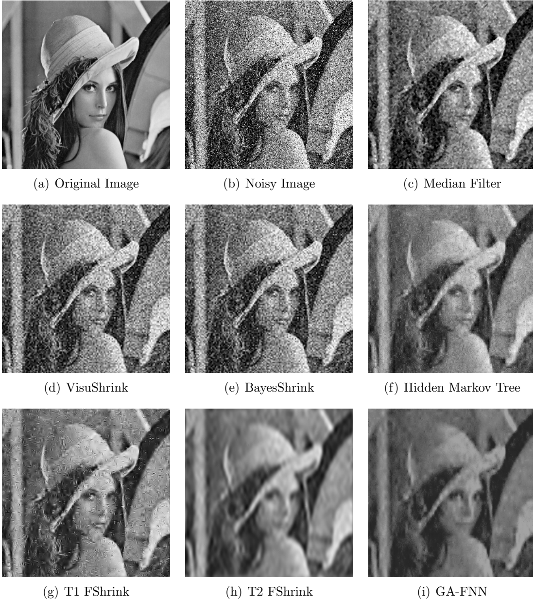
Figure 5.15: Results of “lena” with Gaussian and Impulsive Noise (Both noise variance are 0.05 ). T2 FShrink and GA-FNN outperforms other algorithms. But T2 FShrink blurs the edges in the image.
