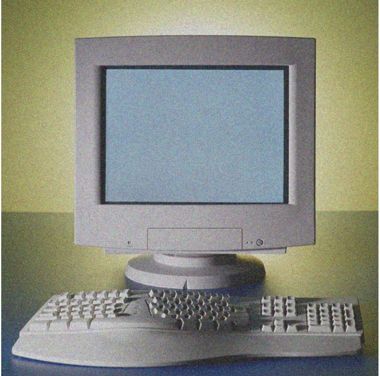
Figure 2.22: Colour image quantized to 3-bits per colour using the nonsubtractive dithering scheme with TPDF dither.
