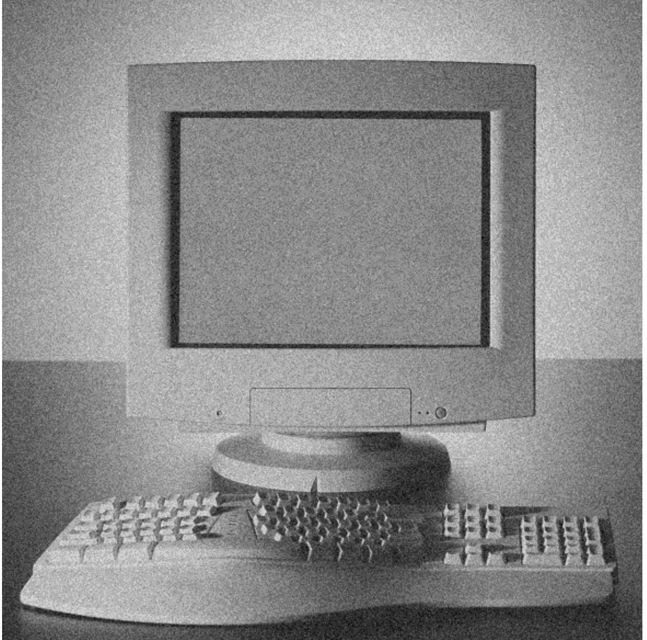
Figure 2.11: Original image quantized to 3-bits using a nonsubtractive dither scheme and TPDF dither.
