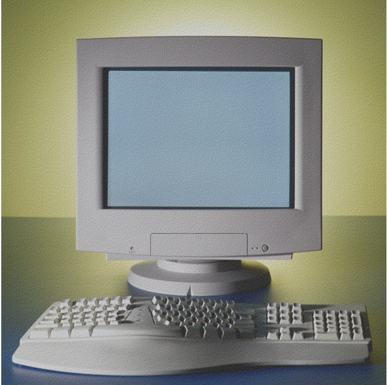
Figure 2.23: Colour image quantized to 3-bits per colour using TPDF dither and the Floyd and Steinberg noise shaper.
