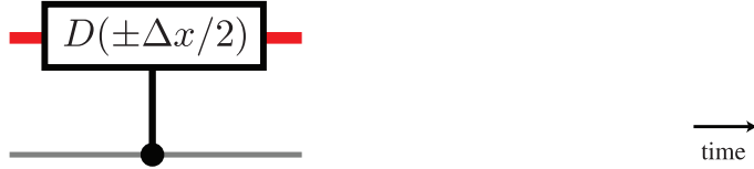
Figure 3.2: Circuit depicting the spatial displacement of a free particle (red line) controlled by the state of a qubit (grey line).
