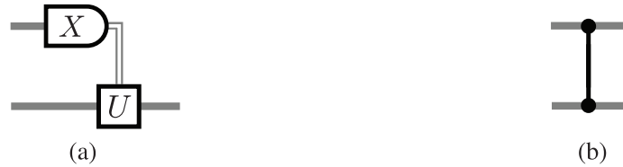
Figure 1: Circuit diagrams depicting (a) projective measurement of a qubit onto the eigenbasis of X with the outcome controlling the application of a unitary U , and (b) the interaction of two qubits via the unitary \wedge Z .
