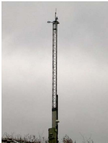
**Figure 3.2: A Typical RWIS Station**
