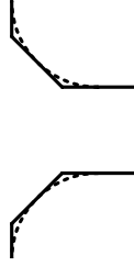
Figure 3.18: Approximating a rounded entrance with a straight, a triangular, and a sudden area change
