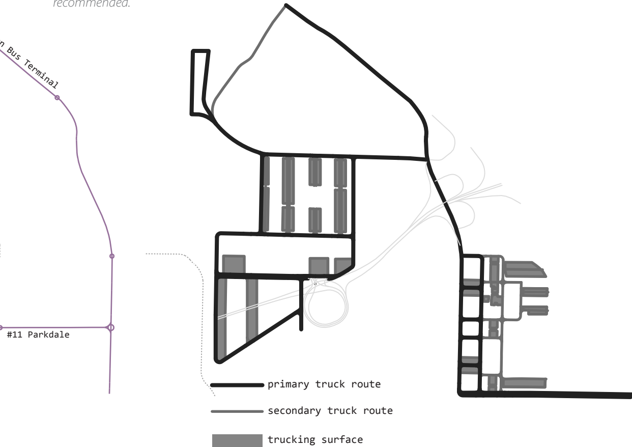
fig. a1.5 Trucking networks — As the park is adapted to new manufacturing uses, new routes for trucks will be integrated with other modes of mobility.
