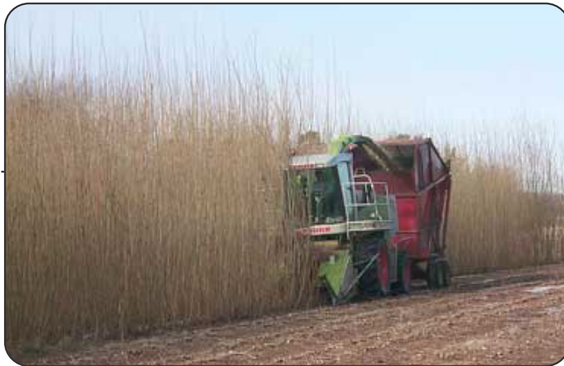
fig. 4.60 Image of specialized high efficiency combine Harvesting willow crops
