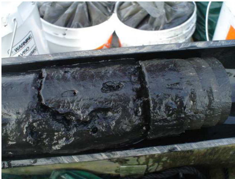
fig. 1.45 Typical sediment core sample taken from Windermere Basin. A 2006 consultant report indicates that the basin is now brought up to a healthy enough state to support aquatic plants.
