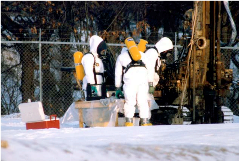
fig. 1.31 Engineers drilling out a soil sample to check its condition at Bruin Lagoon, which was contaminated with heavy metals, sulfuric acid, and crude oil waste. Protective suits are worn to prevent exposure suspected of carcinogens and endocrine disrupters.
