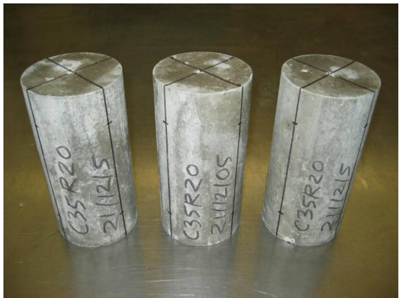
100D×200H mm de-moulded cylinders
