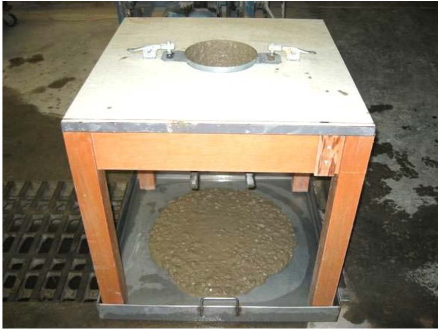
No signs of segregation in inverted slump cone flow spread (C50R0A6)
