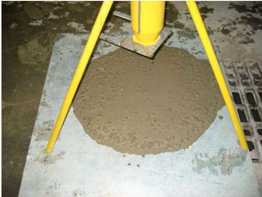
Significant mortar halo in orimet flow spread (C35R15A6)
