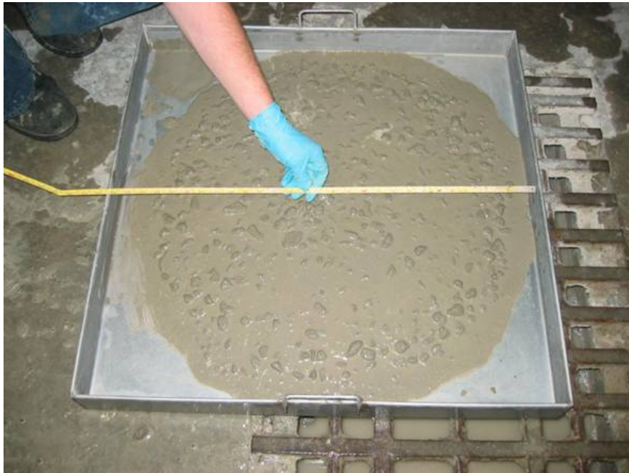
Severe mortar halo in slump flow spread (C35R25A6)
