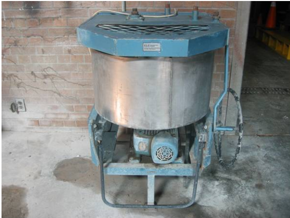
Pan mixer used for preparing concretes
