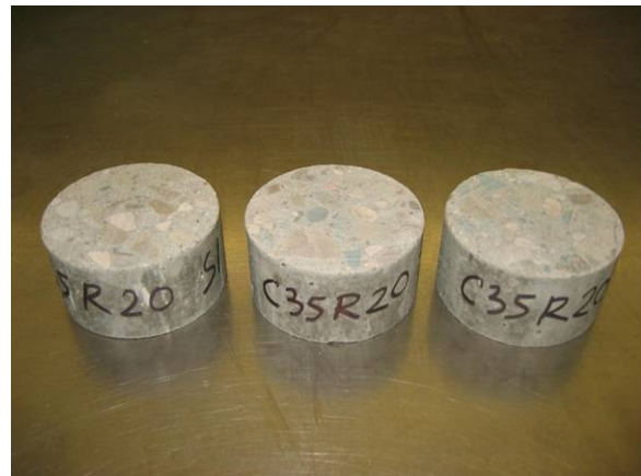
100D×50H mm cut cylinders
