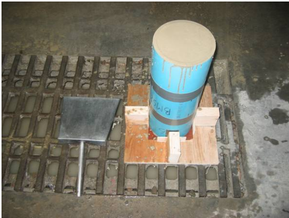
Separator pan and segregation testing in 150D×450H column
