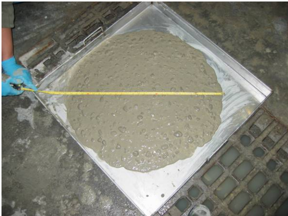
Measurement of slump flow
