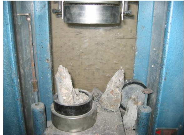
Compression test (after failure)
