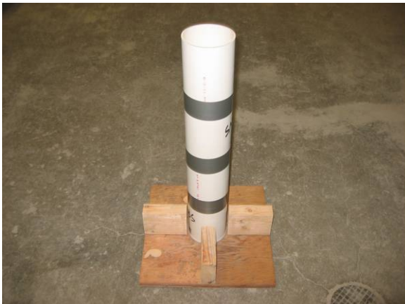
100D×600H columns with 4 sections
