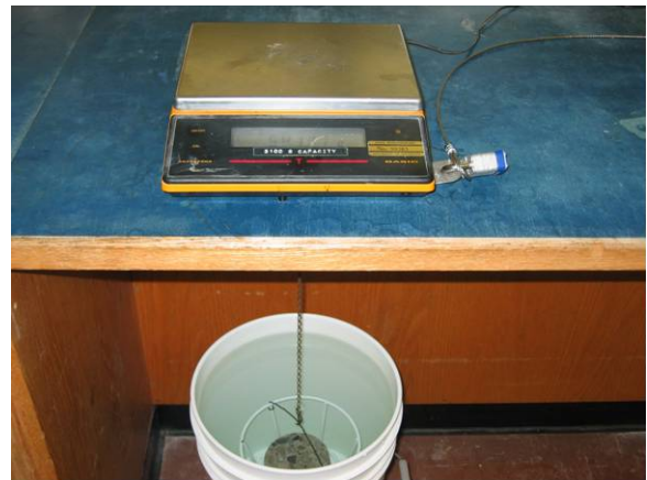
Water absorption and total porosity test (determination of buoyant mass)
