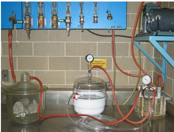
Water absorption and total porosity test (vacuum saturation)
