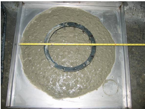
Measurement of slump flow with J-ring
