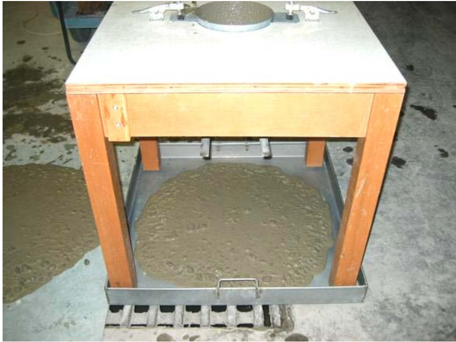
Significant mortar halo in inverted slump cone flow spread (C35R15A6)
