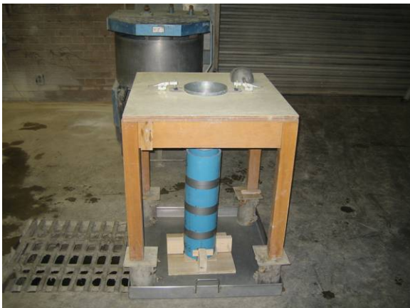
Inverted slump cone used for filling
