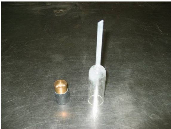
Chace indicator used for determining the air content of mortars
