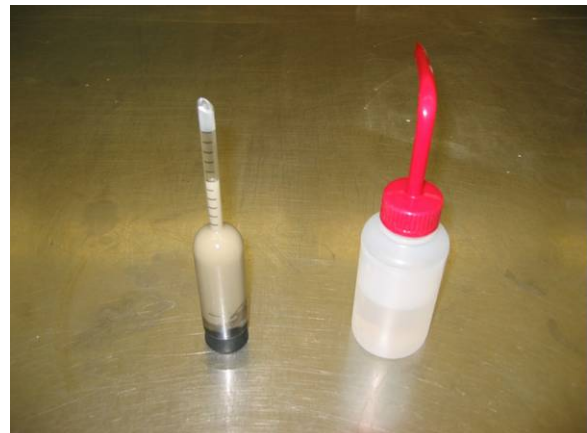
An operational stage to determine the air content of mortars
