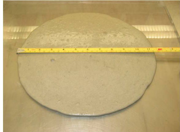
An operational stage to determine the flow spread of mortars
