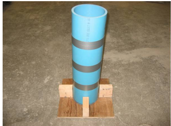
150D×600H columns with 4 sections
