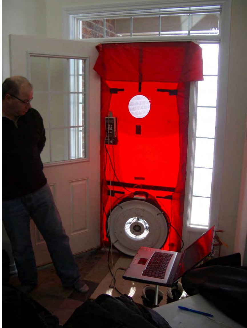
Figure 4.10 – Blower door test setup
