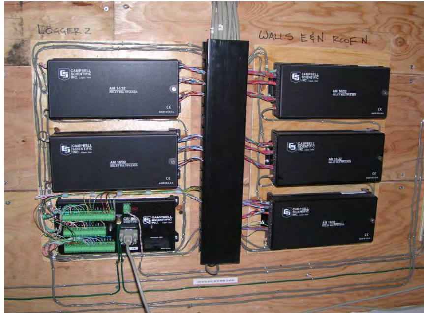
Figure 5.33 – One of two logging and control modules that make up the monitoring system
