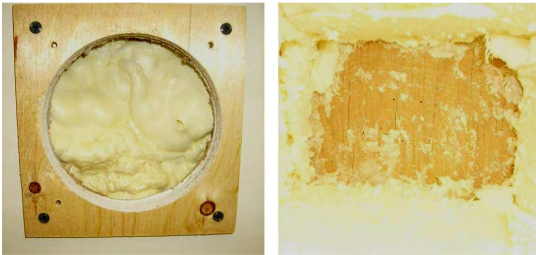
Figure 5.28 – Jig & core through drywall (left) and foam cut to interior face of plywood (right)
