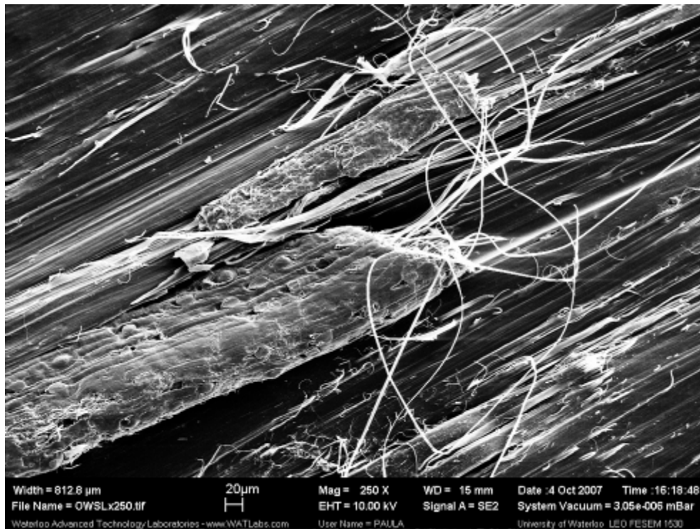
Figure A1.22: 250x mag oriented WS-PP profile, side surface of left profile cross section. Embedded wheat straw.
