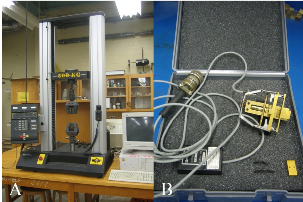
Figure 51: Tensile test apparatus; A - Instron tensile tester; B - Strain gauge
