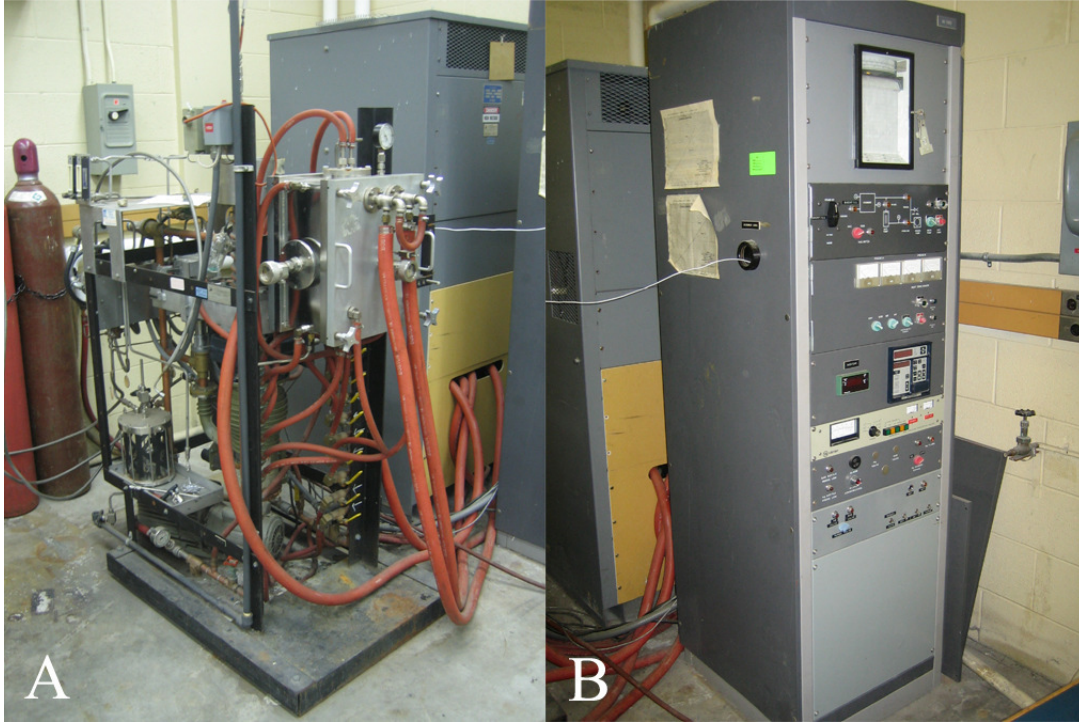
Figure 28: Vacuum furnace. A - chamber, heater, and diffusion pump. B – controller.
