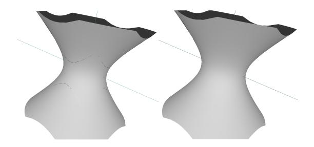
Figure 5.3: A comparison between a stitched tessellation (left) and standard tessellation (right).
