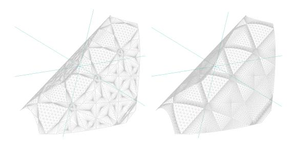
Figure 5.2: A comparison between a standard and adaptive tessellation.
