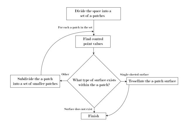
Figure 1.1: The A-patch tessellation algorithm.
