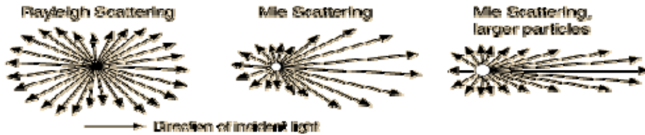
Figure 1.4: Examples of the scattering pattern from three different sizes of aerosol particles 16
