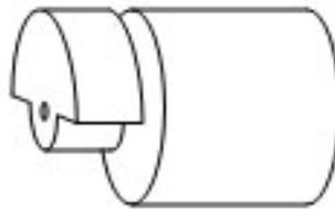
**Figure 5: A DC motor with an attached eccentric rotating mass. Image source: Haywood and MacLean (2007).**
