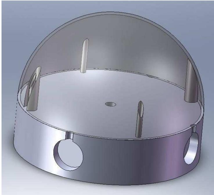
**Figure 16: Hard shell prototype (not shown: tactors and wires).**
