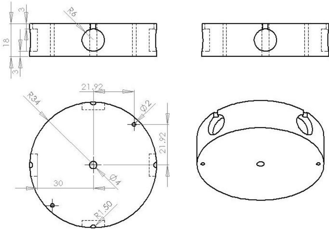
**Figure 26: CAD drawing of PVC disk for hard shell prototype.**
