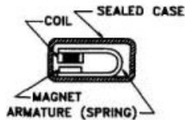
**Figure 4: An inertial transducer. Image source: Cholewiak and Wollowitz (1992).**
