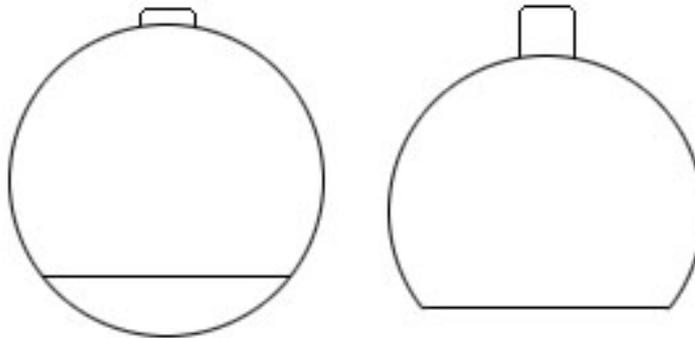
**Figure 1: Simplified view of the veBall in rotation mode (left) and translate/zoom mode (right)**
