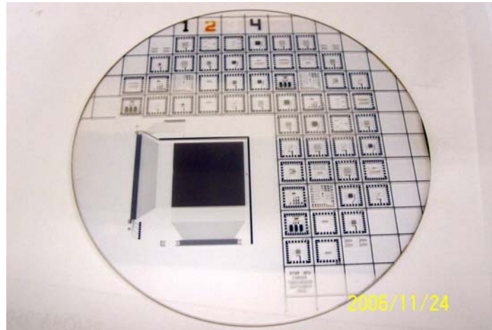
Fig. 4.11. Fabricated thin film circuits on a 3” corning glass wafer.
