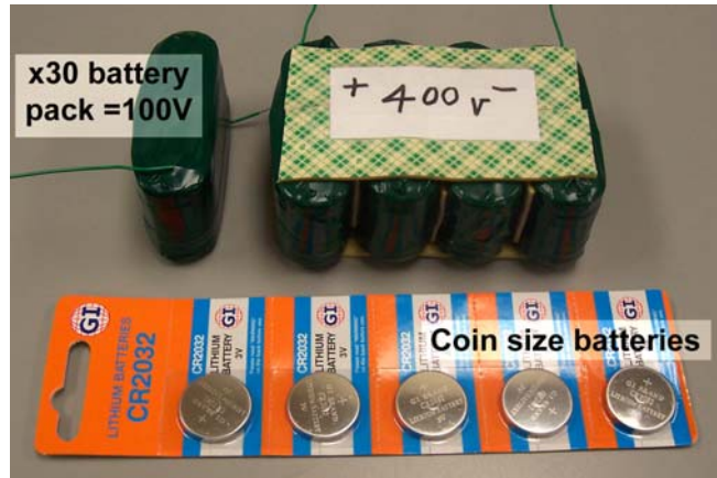
Fig. 5.2. A 400V DC voltage source made up of small 3.3V coin batteries.
