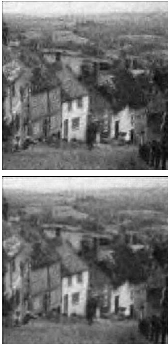
Figure 5.16: (Top) BayesShrink Wavelet Denoising, SNR = 11.59. (Bottom) BayesShrink Wavelet-Ridgelet, SNR = 11.82.
