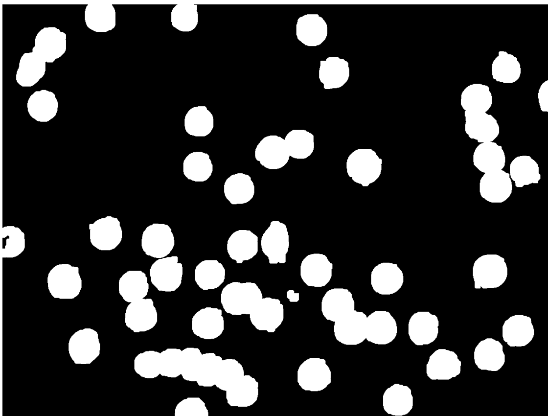
Figure 6.45: Dilating the edge image in (Fig. 6.44) by a disk.
