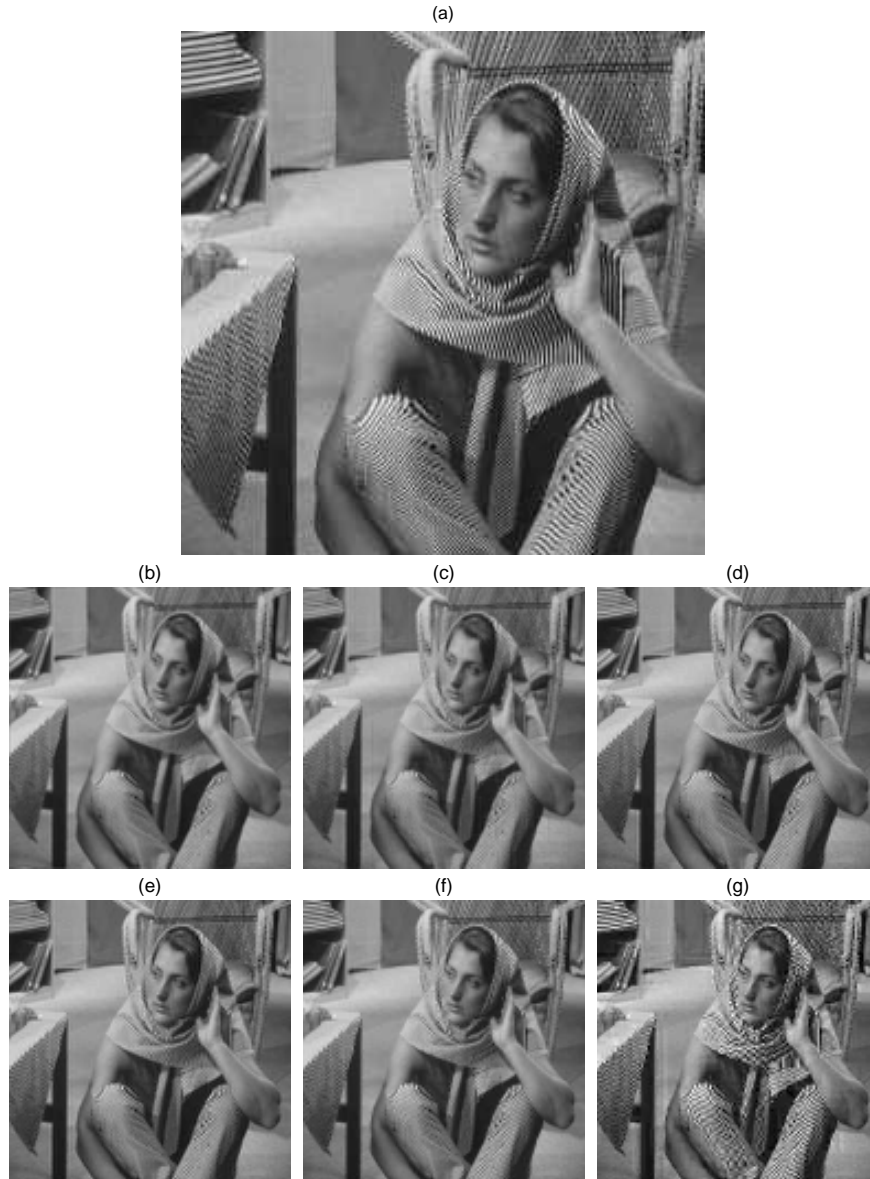
Figure 6.10: Downsampling “Barbara” by 2:1 using six methods: (b) the pre-selected spatial domain method with Butterworth low pass filtering and cubic B-spline interpolation, (c) our method obtained by solving (6.12) with ( d_0 = w_0 = 0.1 ), (d) the method in [12], (e) the M/L method in [58], (f) the bilinear interpolation method in [53], and (g) a fast approximate algorithm with bilinear interpolation in [53]. (a) is the original image with full resolution. Compare the down-sampled images and pay attention to the strips on the top-left corner and the knees. Due to the lack of low-pass filtering in the bilinear interpolation method, slight aliasing is observed in the image of (f), e.g., the erroneous pattern at the left-top corner and the pepper noise at the knees. The image of (g) shows severe aliasing and artifacts.
