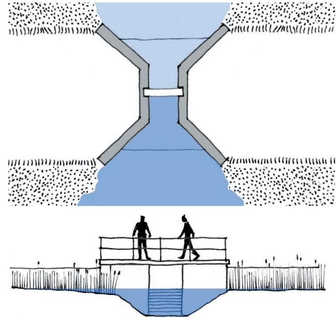
Fig. 139, 140 | Stoplog dams are simple and affordable and allow changes in waterlevel that are required by the various communities in the wetland (see below)
