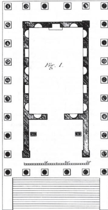
Fig. 6 | Plan of the Temple of Concord and Virtue
