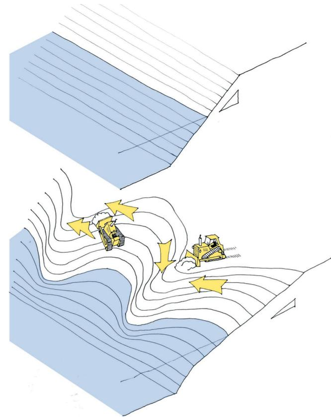
Fig. 130 | Heavy earth moving equipment will sculpt the shoreline to provide earth sheltering and privacy for cottages, enhance the water retention capacity of the terrain, and create a variety of on-shore and shoreline conditions.
