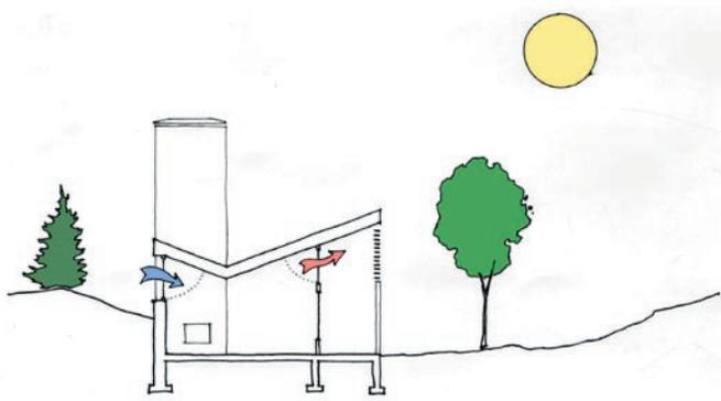
Fig. 141 | Summer shading diagram. Bris-soleil and deciduous plantings on the south side of the cottage provide shade. Generous operable windows allow cross ventilation. Thermal mass created by earth sheltering helps keep the cottage cool
