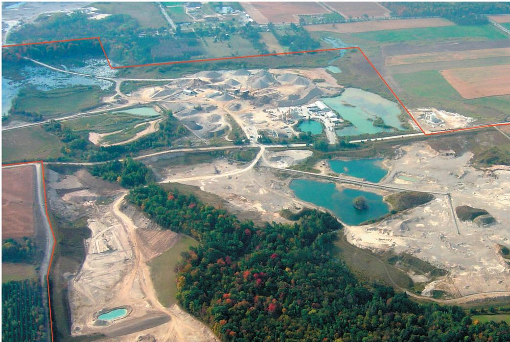
Fig. 62 | The opacity of the ponds is caused by suspended mineral sediment, and not chemical contamination
