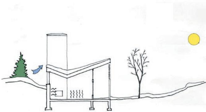
Fig. 142 | Winter heating diagram. The north facing windows can be shuttered and earth sheltering and coniferous plantings help reduce heat loss. Roof pitch corresponds to the end of the cooling season. Deciduous trees drop their leaves and allow low light to penetrate. Thermal mass retains heat from solar gain.
