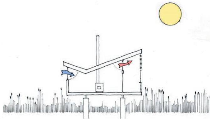
Fig. 146 | Summer shading diagram. Bris-soleil on the south side of the cottage provide shade. Generous operable windows allow cross ventilation.
