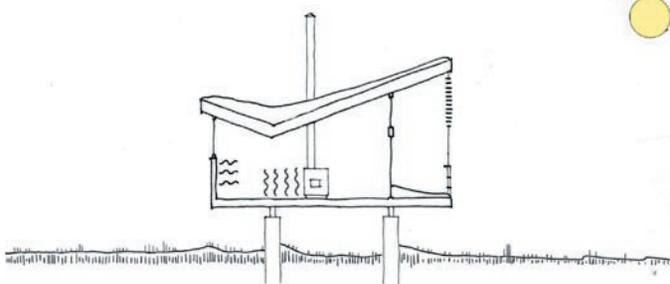
Fig. 147 | Winter heating diagram. The north facing windows can be shuttered to prevent heat loss. Roof slope allows sunlight to penetrate, surfaces absorb heat during the day to be radiated at night.
