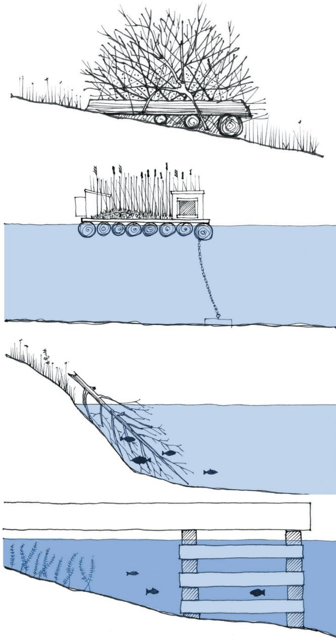
Fig. 152 - 155 | Various types of man-made shelter for animals and fish: brush piles, floating islands, trees and branches acting as fish-cover, docks also provide shelter for fish.
