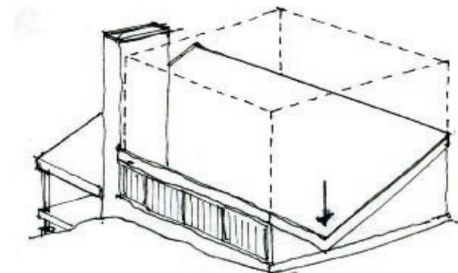
Fig. 145 | Catchment area for rainwater, to be stored in interior cistern
