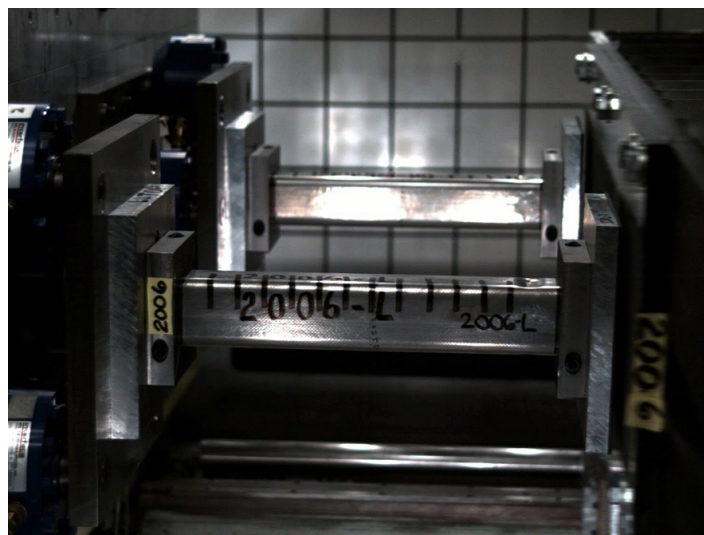
Figure 2.11: Two axial crush specimens mounted on sled-track
