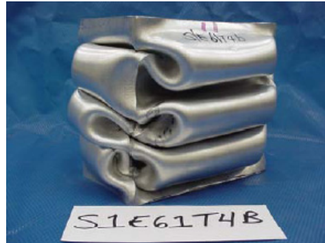
Figure 1.6: Deformation of 6061-T4 aluminum tube [13]
