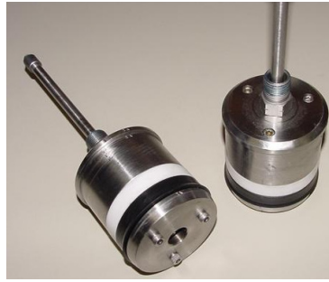
Figure 2.8: End-plugs used to seal tubes during hydroforming without end-feeding
