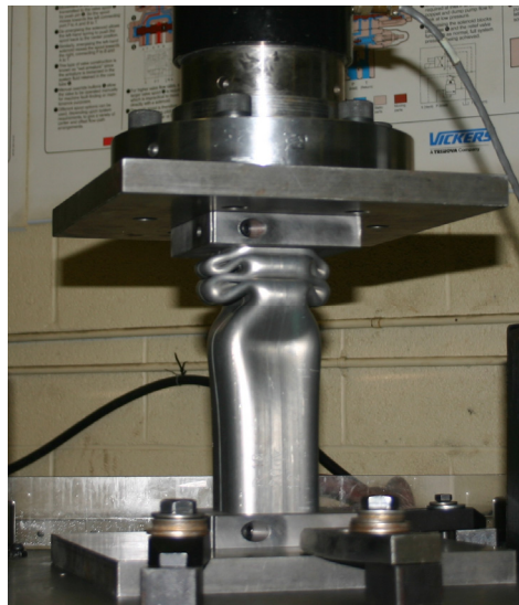
Figure 2.13: Experimental set-up for quasi-static axial crush testing
