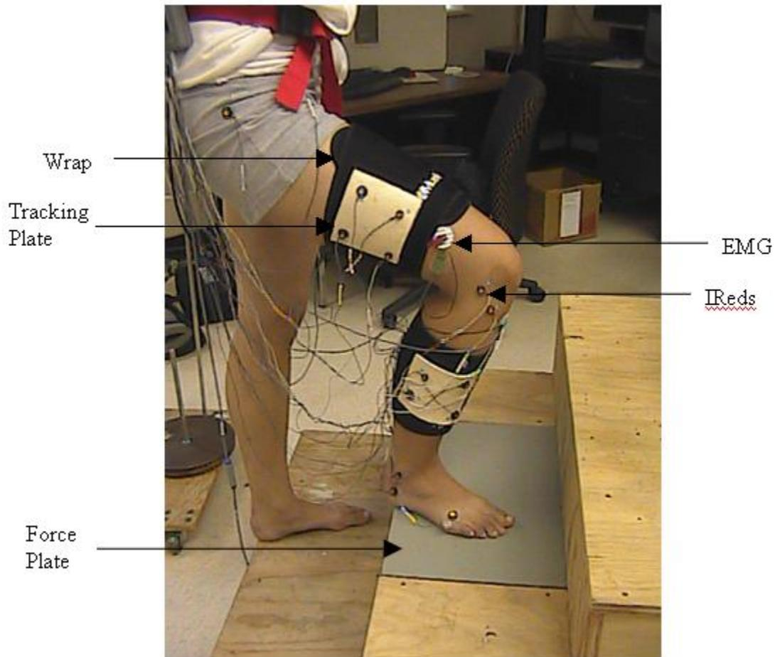
**Figure 4.3:** *Experimental setup for the data collection. The force plate is embedded into the second step. The tracking plates, both on the thigh and shank were secured to the wraps with Velcro. The EMG was located under the neoprene wraps; one of the two electrodes was exposed. The IReds (motion markers) can be seen on the knee joint, foot, hip and tracking plates.*
