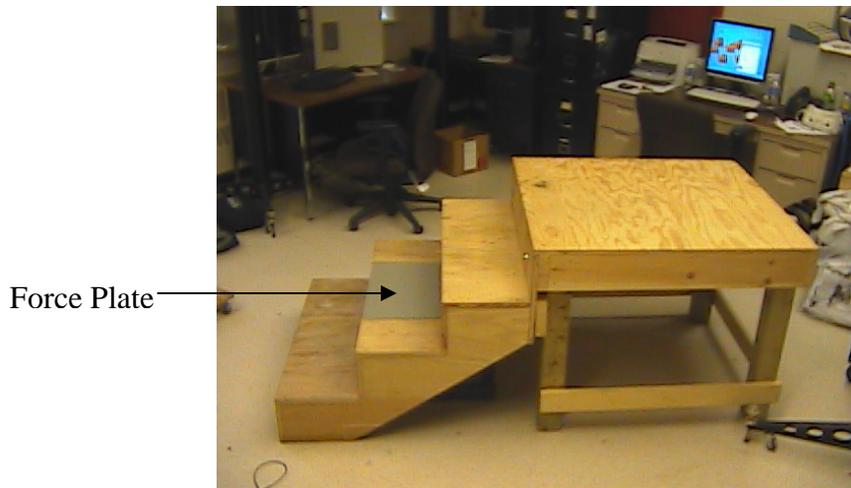
**Figure 4.2:** Staircase used for the ascent and descent trials. Rise = 20cm. Run = 30cm.
