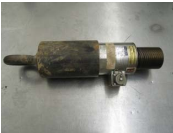
Figure 5-16: External Load Cell used to measure Pullout force applied to Carrier Casing.
