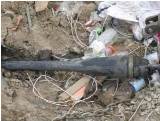
Figure 6-18: Reduced Diameter in 100-mm Perforated Pipe after Last Attempt
