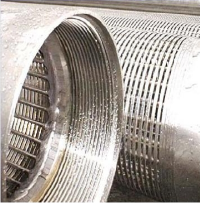
Figure 4-2: Stainless Steel Well Screen for the 2 nd Field Trial (Cox et al 2000)
