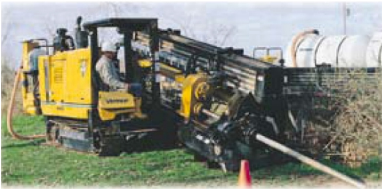
Figure 3-4: Midi-HDD Rig (Vermeer Manufacturing Company 2004)
