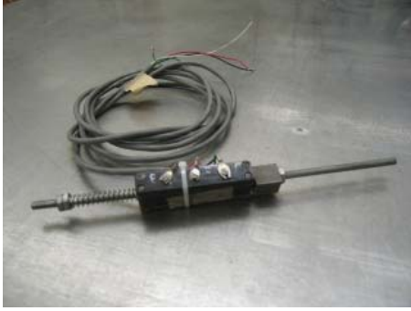
Figure 5-11: Displacement Transducer used to monitor carrier casing wall deflections.
