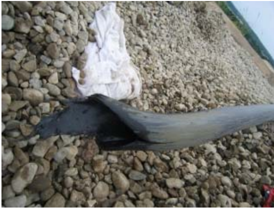
Figure 6-17: Failure of 100-mm OD HDPE Well Pipe during 4 th Attempt
