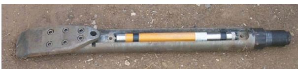
Figure 3-9: Sonde location inside the Drill Head (HDD Consortium 2001).
