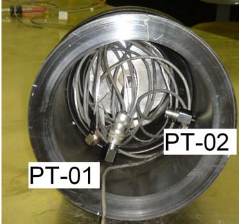
Figure 5-14: East Well HDPE carrier casing Pressure Transducers location.
