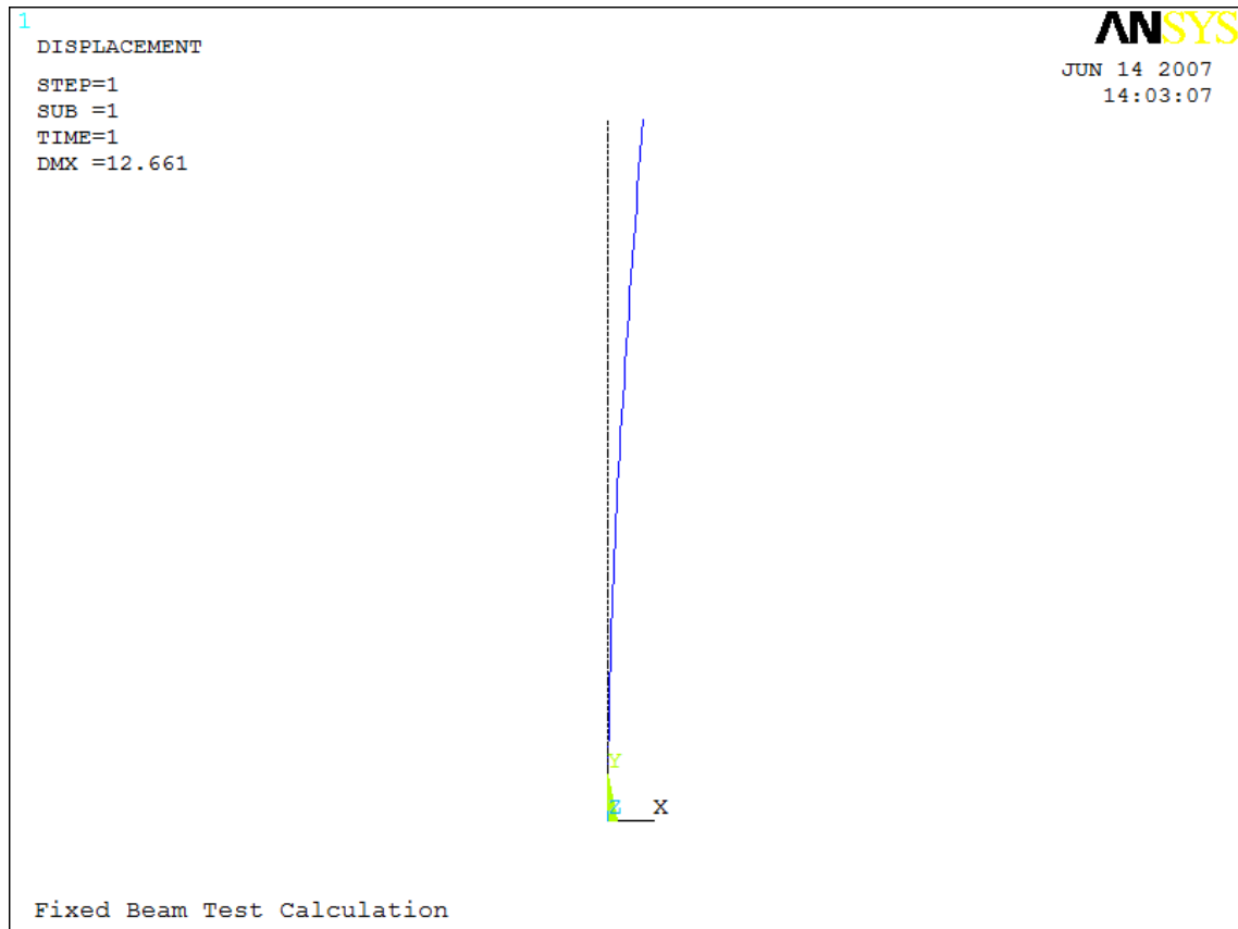
Figure 4.4: Fixed beam with perpendicular point force of 1 \mu\text{N} to yield a displacement of 12.66 \mu\text{m} in the direction of the force.
