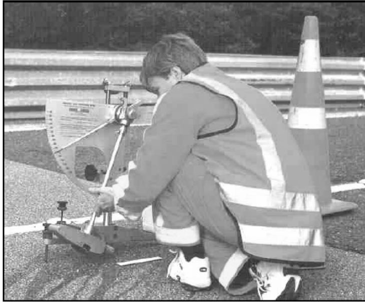
Figure 2.18: British Pendulum Tester (BPT) in use [Henderson 06]
