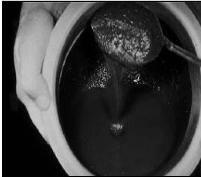
Figure 2.28: Photograph illustrating good mixture consistency [Caltrans 03]
