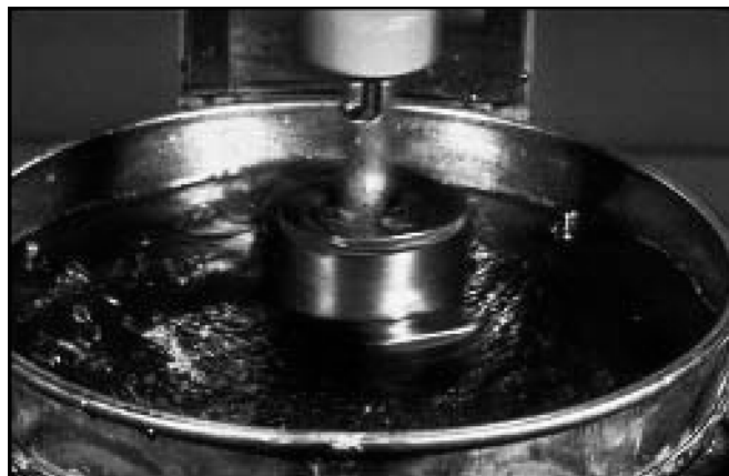
Figure 2.29: Orbital grinding of sample using rubber hose attachment [Caltrans 03]
