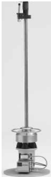
FIGURE G-6 Assembled PFWD Device
