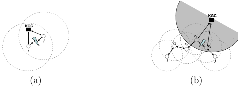
Figure 6.3: Active Attacks in Model I with: (a) one-hop communication between nodes i and j , (b) multi-hop communication between nodes i and j .
